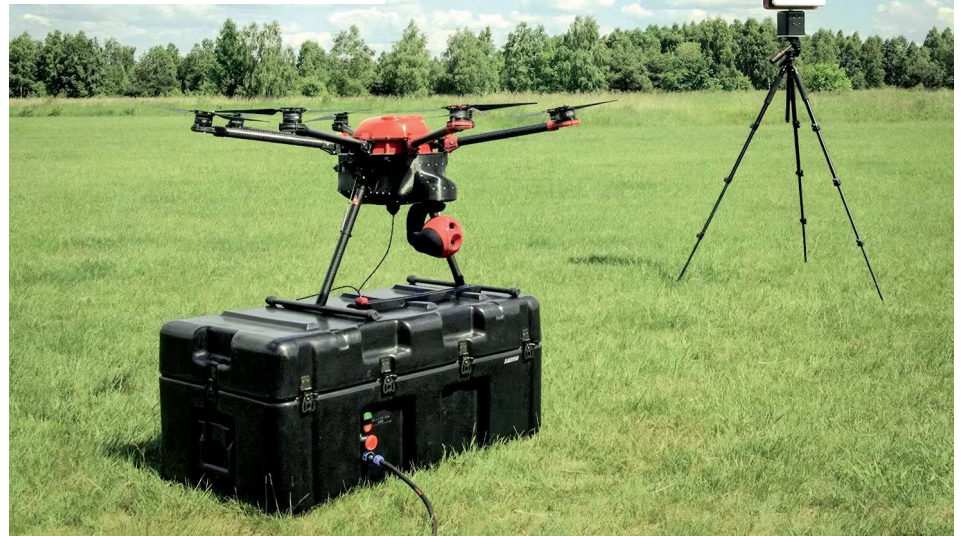
A tethered UAV with ground-based power management systems (Courtesy of Vicor)
