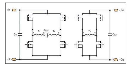
Figure 3: Simplified schematic of the Pre-Regulator Module
