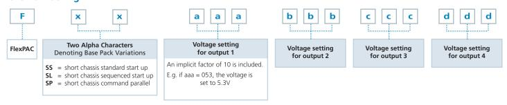
FSS103-205-033-000 is a short chassis standard start up FlexPAC with 3 outputs set at 10.3V, 20.5V, and 3.3.V Pg
