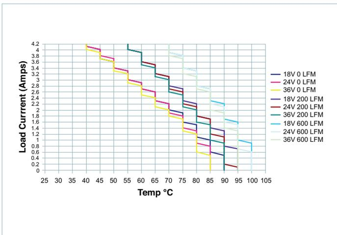
Figure 12 — Load current vs. temperature (without heat sink)
