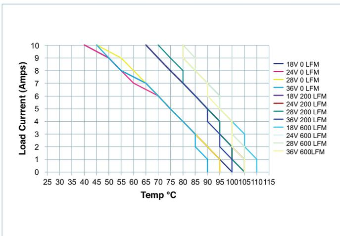
Figure 3 — Load current vs. temperature (6.3mm heat sink)
