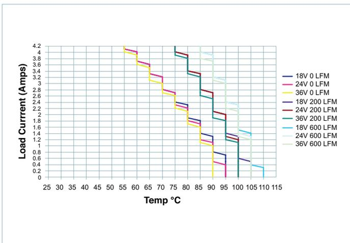
Figure 13 — Load current vs. temperature (6.3mm heat sink)
