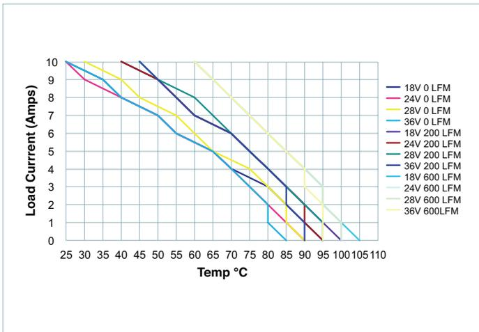
Figure 2 — Load current vs. temperature (without heat sink)
