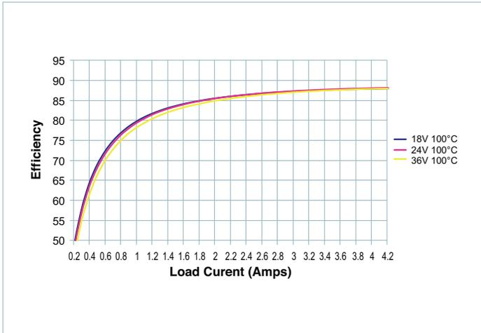
Figure 11 — Conversion efficiency
