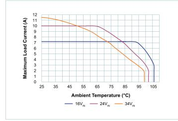
Figure 18 — Thermal de-rating @ V<sub>OUT</sub> = 12V
