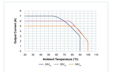
**Figure 22** — Thermal de-rating @  $V_{OUT} = 34V$  with Limited Input Range ( $24V_{IN}$  to  $34V_{IN}$ )
