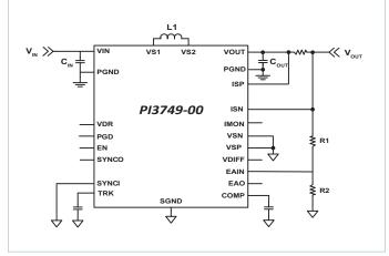
Figure 24 — ZVS Buck-Boost with required components
