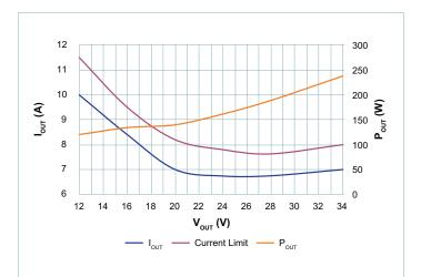
Figure 16 — Power and current output at 24V<sub>IN</sub>
