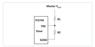
Figure 26 — Voltage divider connections for direct tracking
