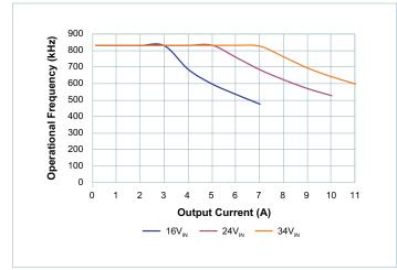
Figure 7 — Switching Frequency vs. Output Current @ 12V<sub>OUT</sub>
