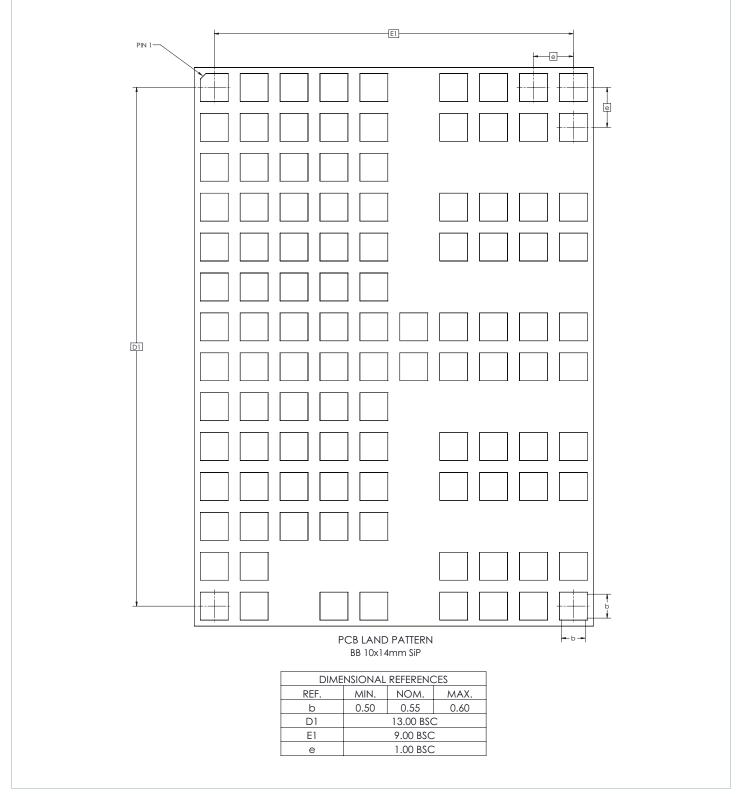
Recommended receiving footprint for PI3749-x0 10mm x 14mm package. All pads should have a final copper size of 0.55mm x 0.55mm, whether they are solder-mask defined or copper defined, on a 1mm x 1mm grid. All stencil openings are 0.45mm when using either a 5mil or 6mil stencil.
