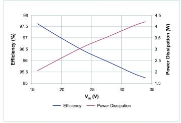
**Figure 12** — 12V<sub>OUT</sub> Efficiency and Power Dissipation at 7A over Input Voltage Range
