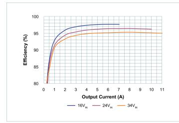
Figure 2 — 12V<sub>OUT</sub> Efficiency
