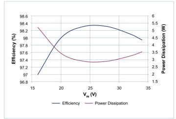
**Figure 14** — 28V<sub>OUT</sub> Efficiency and Power Dissipation at 6A over Input Voltage Range
