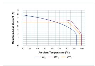
Figure 20 — Thermal de-rating @ V<sub>OUT</sub> = 28V
