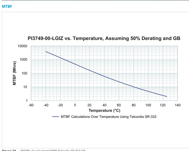
Figure 23 — PI3749-x0 calculated MTBF Telcordia SR-332 GB
