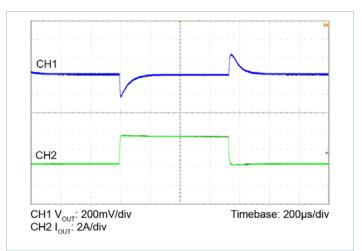
Figure 5 —  $24V_{IN}$  to  $24V_{OUT}$ ,  $C_{OUT} = 8 \times 10 \mu$ F Ceramic 3.0A Load Step at 5A/ $\mu$ s
