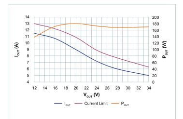
**Figure 15** — Power and current output at  $34V_{IN}$
