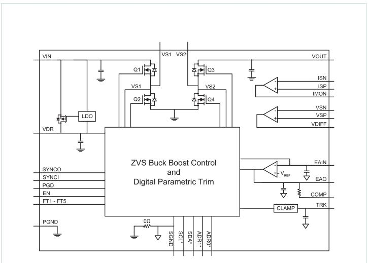
\*Simplified Block Diagram (I<sup>2</sup>C pins SCL, SDA, ADRO, ADR1, only active for PI3749-20 device version)
