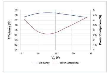
**Figure 13** — 24V<sub>OUT</sub> Efficiency and Power Dissipation at 7A over Input Voltage Range
