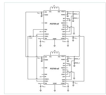
Figure 27 — PI3749-x0 parallel operation
