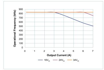
Figure 8 — Switching Frequency vs. Output Current @ 24V<sub>OUT</sub>
