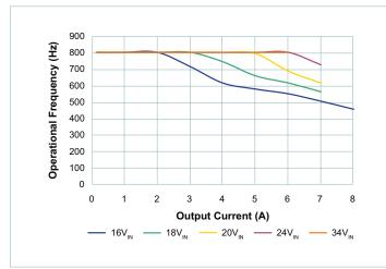
Figure 9 — Switching Frequency vs. Output Current @ 28V<sub>OUT</sub>
