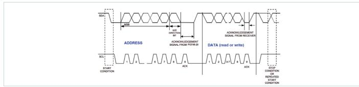
Figure 28 — Data transfer on the  $l^2C$  bus
