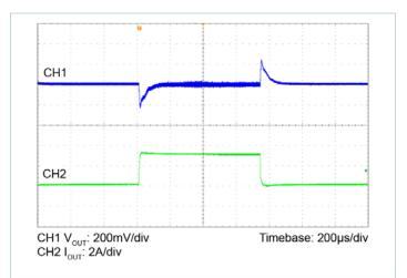
**Figure 6** —  $16V_{IN}$  to  $28V_{OUT}$ ,  $C_{OUT} = 8 \times 10\mu$ F Ceramic 3.0A Load Step at  $5A/\mu$ s
