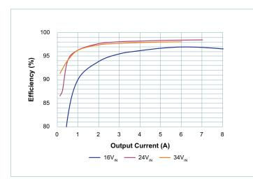
Figure 3 — 28V<sub>OUT</sub> Efficiency
