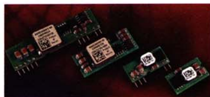
The Austin SuperLynx and MicroLynx families are popular POL converters. Tyco manufactures SMT versions that mount parallel to the host board and through-hole-mounted SIP versions.
