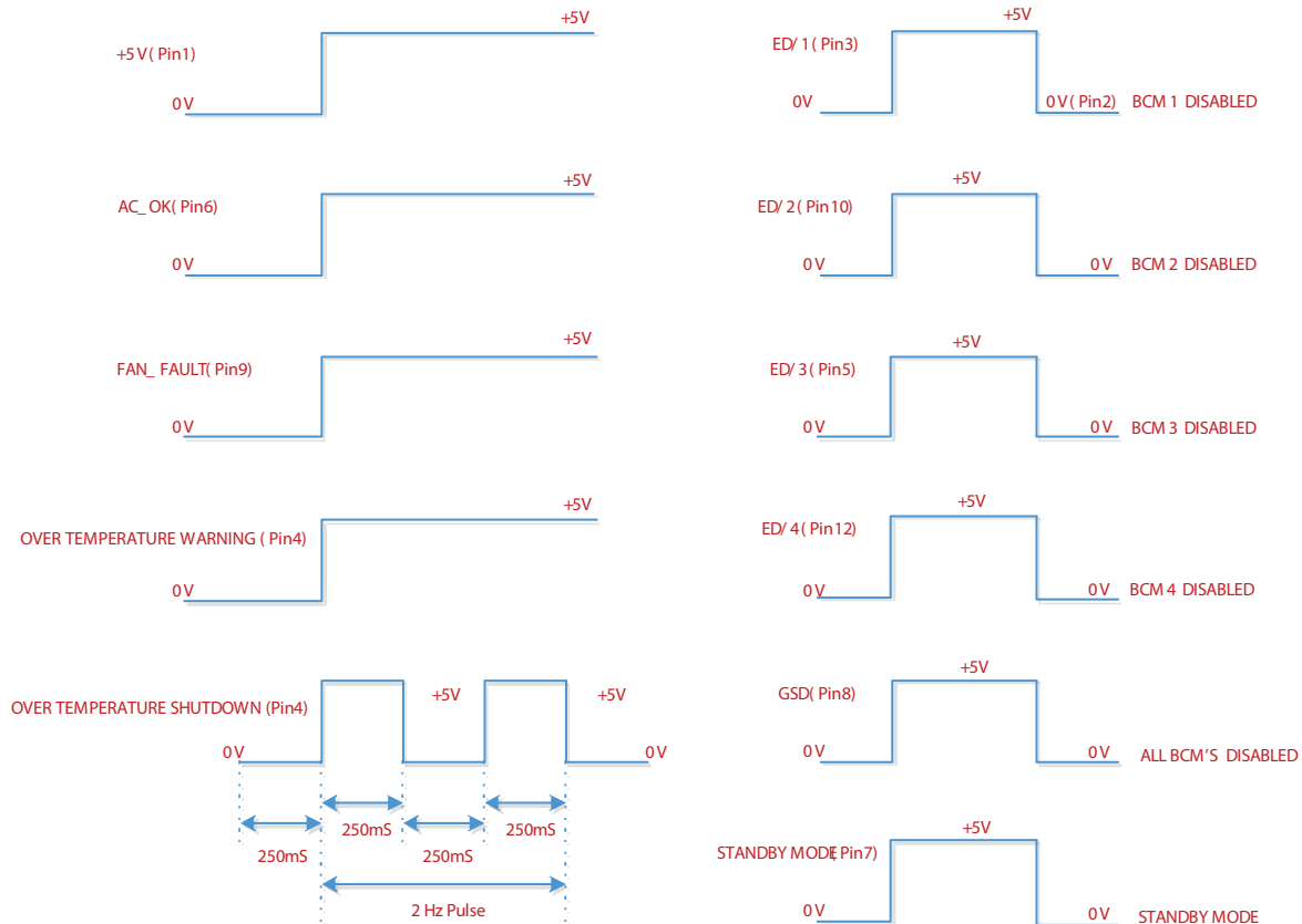
Figure 10. Output TTL logic Signals
