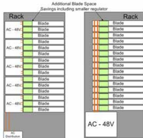
Figure 8: Possible implementations of an AC – 48V – 1.xV architecture
