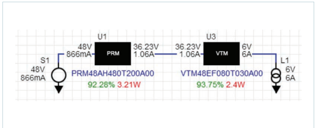
Figure 5 Efficiency calculation, Vicor PowerBench™ whiteboard for supplemental converter
