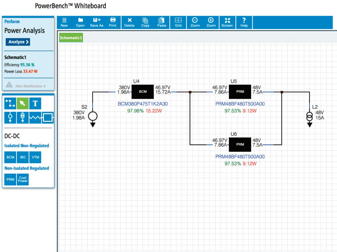
While the PowerBench Whiteboard is an excellent tool for quickly architecting a power system design, Vicor also offers a full featured online simulator which allows a customer to evaluate a component's electrical and thermal performance. The PowerBench Simulator analyzes the converter under a range of situations (startup, steady state,  $V_{IN}$  or load steps) in a typical reference design. Figure 4 shows the simulation tool with the BCM380P475T1K2A30 displayed.
