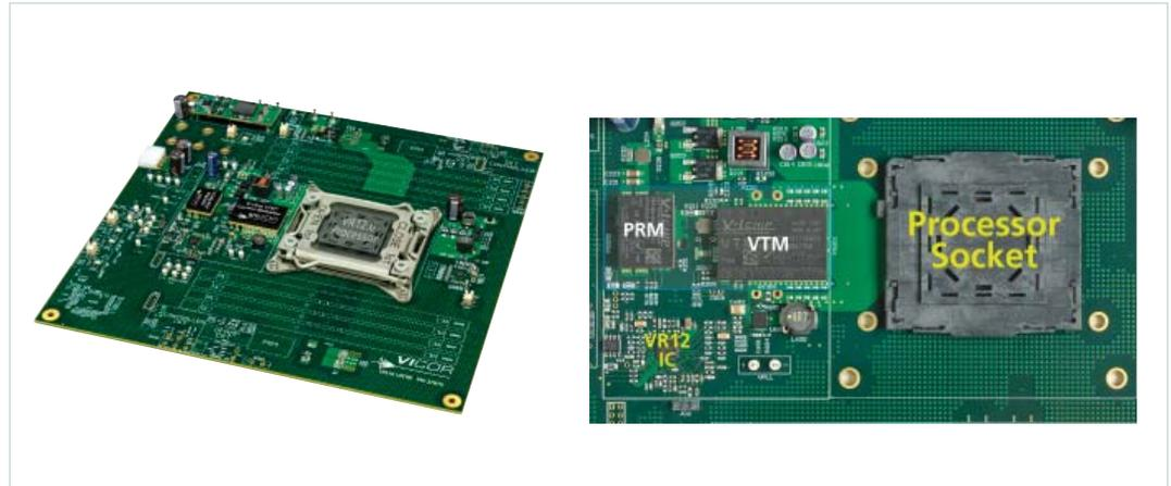
A Voltage Test Tool (VTT) is inserted into the processor socket which emulates processor behavior to characterize the performance of the powertrain. The performance is recorded and compared to the VR12.0 specifications using an automated spreadsheet. A typical 'Load Line' result, in which  $V_{CORE}$  must remain within tight limits while processor current increases, is shown in Figure 6.
