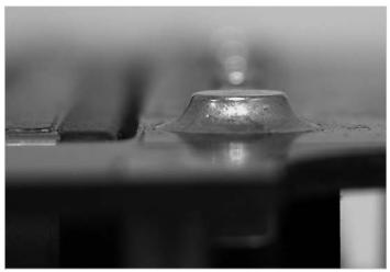
Figure 23.1 — Side profile of a Mini module solder joint
