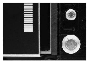
Figure 23.2 — Maxi / Mini output power pin and Sense pin
