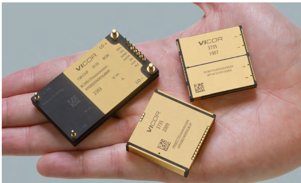
Figure 5: BCM®, PRM™ and DCM™ power modules effectively address safety requirements while delivering high efficiency and minimising space consumption
