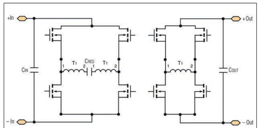
**Figure 3: Simplified schematic of the Pre-Regulator Module**
