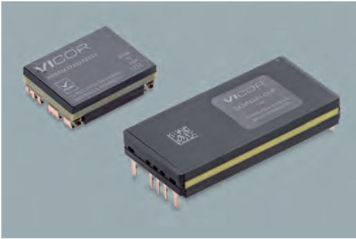
Figure 3: Vicor DCM4623 is power dense and has a safe current-limiting feature for counter-UAS platforms. Vicor DCM™ DC-DC converters are designed to handle large amounts of capacitance at their outputs and can operate within their maximum current rating and power rating even when driving capacitance values as large as 10 millifarads.
