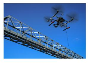
Fukaden's tethered drone launches a communication base station that delivers immediate mobile phone services to support relief efforts of first responders.
