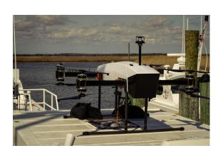
Dragonfly Picture's tethered helicopter drones are an essential element for today's communication and surveillance that can extend maritime radio line of sight from 8 to 30 miles.
