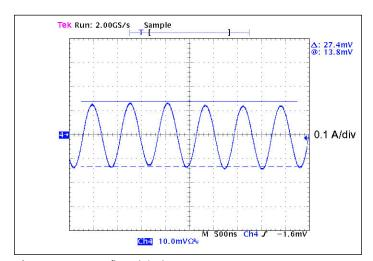
Figure 4 — Input reflected ripple current
