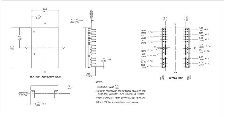
Figure 21 — PRM Through-hole mechanical outline
