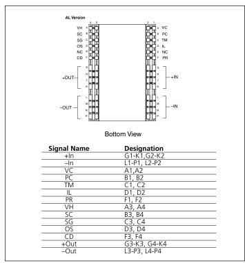
Figure 15 — PRM pin configuration
