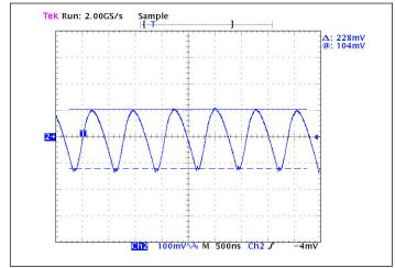
Figure 14 — Output ripple full load 10 μF bypass capacitance
