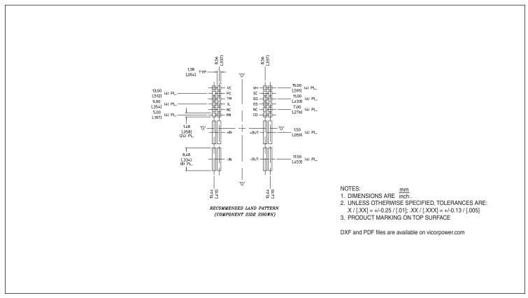
Figure 20 — PRM J-Lead PCB land layout information; Onboard mounting
