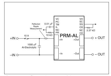
**Figure 5** — Input filter capacitor recommendation
