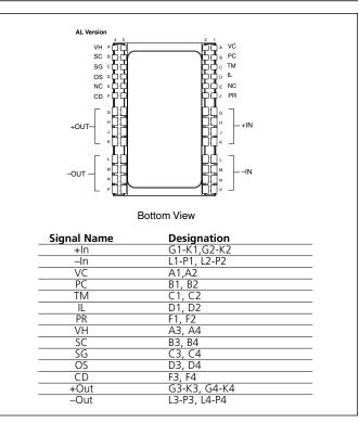
Figure 15 — PRM pin configuration
