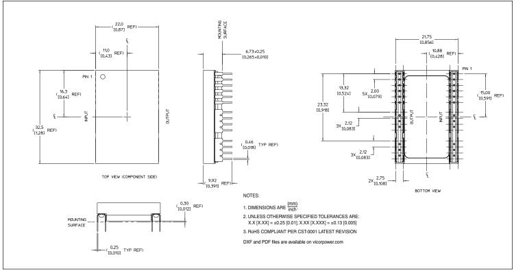
Figure 21 — PRM Through-hole mechanical outline
