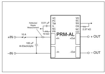
Figure 5 — Input filter capacitor recommendation
