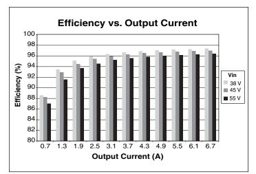
Figure 7 — Efficiency vs. output current at 36 Vf
