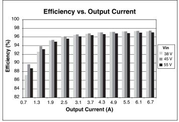
Figure 6 — Efficiency vs. output current at 48 Vf
