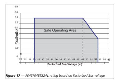
The Factorized Bus voltage should not exceed an absolute limit of 55 V, including steady state, ripple and transient conditions. Exceeding this limit may cause the internal OVP set point to be exceeded.
