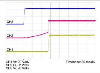
Figure 2 — Vf and PC response from power up
