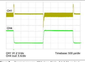
Figure 9 — Transient response; PRM alone 45 Vin, 0-6.7-0A, no load capacitance, local loop
