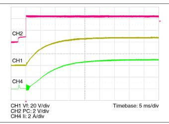
Figure 3 — Vf turn-on waveform with inrush current – PC enabled
