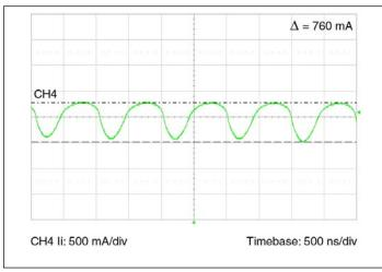
Figure 4 — Input reflected ripple current
