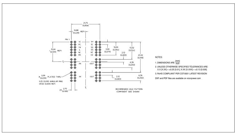
Figure 22 — PRM Through-hole PCB layout information
