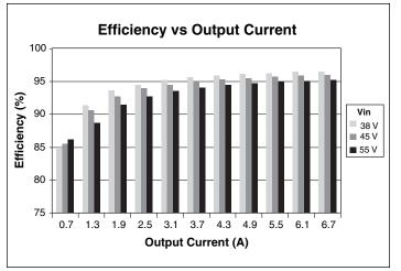
Figure 8 — Efficiency vs. output current at 26 Vf
