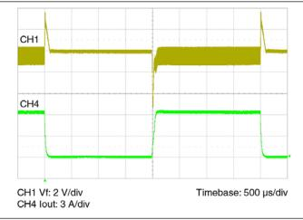
Figure 10 — Transient response; PRM alone 38 Vin, 0-6.7-0A no load capacitance, local loop
