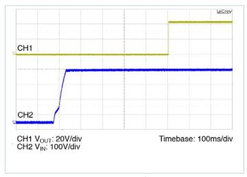
**Figure 13** —  $V_{IN}$  to  $V_{OUT}$  start up wave form
