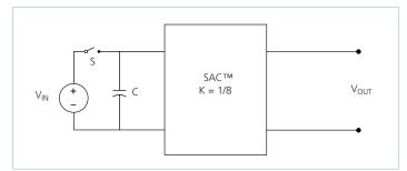
**Figure 20** — Sine Amplitude Converter™ with input capacitor
