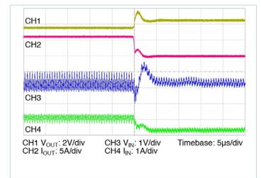
**Figure 14** — 7.7A – 0A transient response:  $C_{IN} = 330 \mu F$ ,  $I_{IN}$  measured prior to  $C_{IN}$ , no external  $C_{OUT}$
