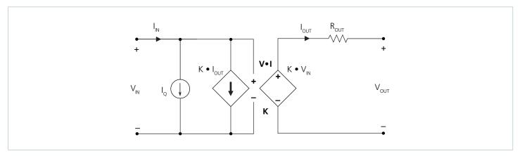
Figure 18 — VI Chip® module DC model
