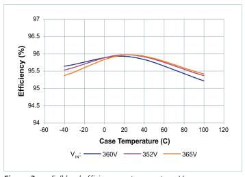
**Figure 3** — Full load efficiency vs. temperature;  $V_{IN}$
