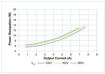
**Figure 9** — Power dissipation at  $T_{CASE} = 100$ °C
