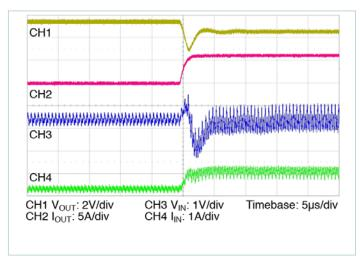
**Figure 15** — 0A - 7.7A transient response:  $C_{IN} = 330\mu F$ ,  $I_{IN}$  measured prior to  $C_{IN}$ , no external  $C_{OUT}$
