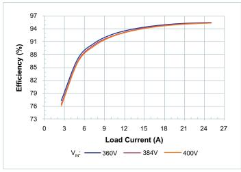
**Figure 5** — Efficiency at  $T_{CASE} = -40$ °C
