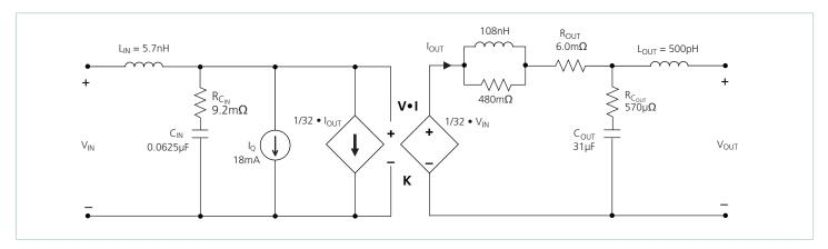
Figure 17 — VI Chip® module AC model
