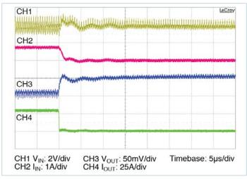
**Figure 16** — 27.3A – 0A transient response:  $C_{IN} = 1\mu F$ ,  $I_{IN}$  measured prior to  $C_{IN}$  no external  $C_{OUT}$
