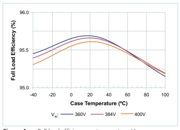
**Figure 4** — Full load efficiency vs. temperature;  $V_{IN}$
