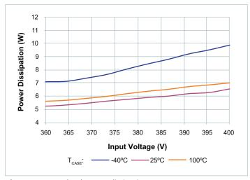
**Figure 3** — No load power dissipation vs.  $V_{IN}$
