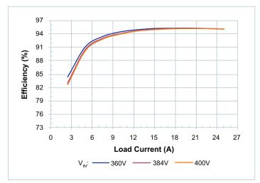
**Figure 9** — Efficiency at  $T_{CASE} = 100$ °C
