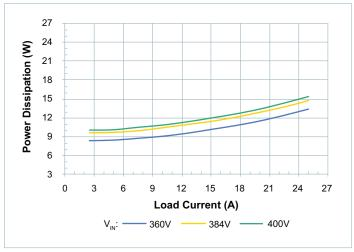
**Figure 6** — Power dissipation at  $T_{CASE} = -40$ °C
