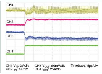
**Figure 15** — 0A - 27.3A transient response:  $C_{IN} = 1\mu F$ ,  $I_{IN}$  measured prior to  $C_{IN}$ , no external  $C_{OUT}$
