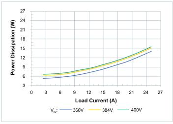
**Figure 10** — Power dissipation at  $T_{CASE} = 100^{\circ}C$
