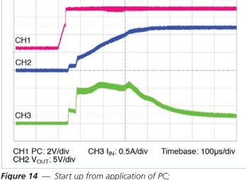
**Figure 14** — Start up from application of PC,  $V_{IN}$  pre-applied  $C_{OUT} = 1000 \mu F$
