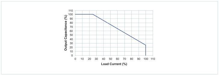
Figure 2 — Start up load current vs. output capacitance
