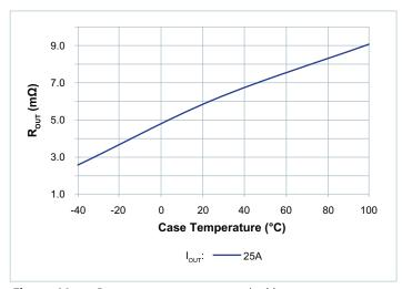
**Figure 11** — R<sub>OUT</sub> vs. temperature; nominal input
