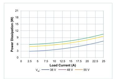
**Figure 7** — Power dissipation at  $T_{CASE} = 25^{\circ}C$
