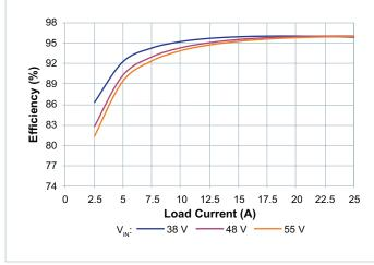
**Figure 6** — Efficiency at T<sub>CASE</sub> = 25°C
