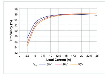
**Figure 8** — Efficiency at T<sub>CASE</sub> = 100°C
