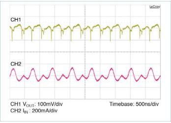
**Figure 12** — Full load ripple,  $330\mu$ F C<sub>IN</sub>: No external C<sub>OUT</sub>, Board mounted module, scope setting : 20MHz analog BW
