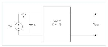
Figure 18 — Sine Amplitude Converter<sup>TM</sup> with input capacitor
