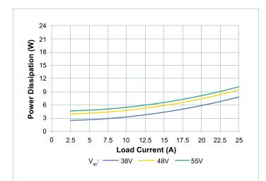
**Figure 9** — Power dissipation at  $T_{CASE} = 100^{\circ}C$
