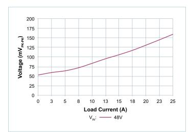
**Figure 11** — V<sub>RIPPLE</sub> vs. I<sub>OUT</sub>: No external C<sub>OUT</sub>, board mounted module, scope setting : 20MHz analog BW
