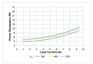
**Figure 7** — Power dissipation at  $T_{CASE} = 25$ °C
