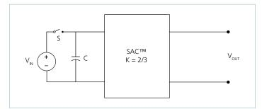
Figure 18 — Sine Amplitude Converter™ with input capacitor
