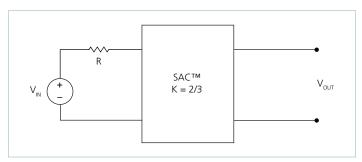
**Figure 17** — K = 2/3 Sine Amplitude Converter with series input resistor
