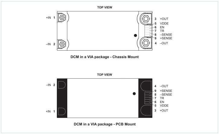
Note: The dot on the VIA housing indicates the location of the control pin 9 (+SENSE pin).
