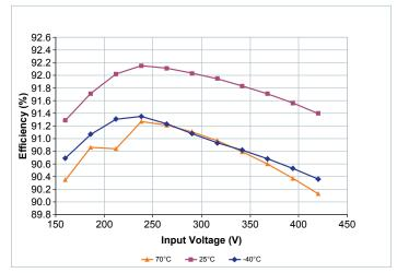
Figure 8 — Full Load Efficiency vs. V<sub>IN</sub>, at nominal trim
