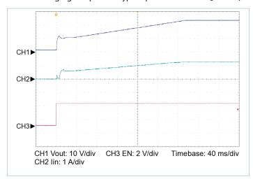
**Figure 15** —Startup from EN,  $V_{IN}$  = 270 V,  $C_{OUT\_EXT}$  = 2200  $\mu$ F,  $R_{LOAD}$  = 1.152  $\Omega$
