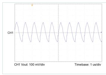
Figure 17 — Output voltage ripple,  $V_{IN}$  = 270 V,  $V_{OUT}$  = 24.0 V,  $C_{OUT\_EXT}$  = 220  $\mu$ F,  $R_{LOAD}$  = 1.152  $\Omega$
