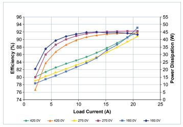
**Figure 11** — Efficiency (top three curves) and power dissipation (bottom three curves) vs.load at  $T_{CASE} = 25^{\circ}C$ , nominal trim
