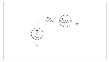
Figure 19 - Single-sided cooling VIA thermal model
