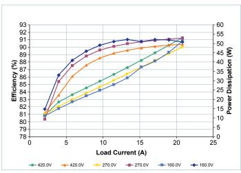
**Figure 10** — Efficiency (top three curves) and power dissipation (bottom three curves) vs.load at  $T_{CASE} = -40^{\circ}C$ , nominal trim
