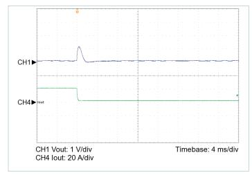
**Figure 5** — 100% to 10% load transient response,  $V_{IN}$  = 270 V, nominal trim,  $C_{OUT\_EXT}$  = 220  $\mu$ F
