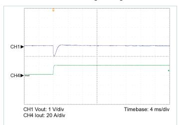
**Figure 6** — 10% to 100% load transient response,  $V_{IN}$  = 270 V, nominal trim,  $C_{OUT\_EXT}$  = 220  $\mu$ F
