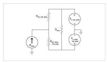
Figure 18 – Double sided cooling VIA thermal model
