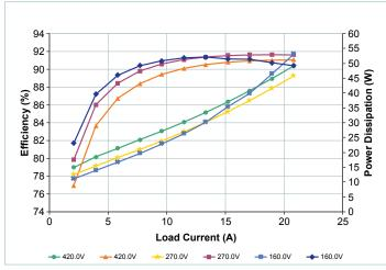
**Figure 12** — Efficiency (top three curves) and power dissipation (bottom three curves) vs.load at  $T_{CASE} = 70^{\circ}$ C, nominal trim
