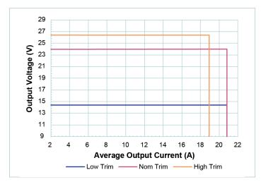
Figure 2 — Electrical Specified Operating Area
