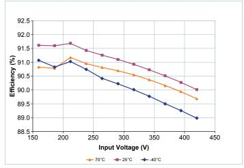
Figure 7 — Full Load Efficiency vs. V<sub>IN</sub>, at low trim
