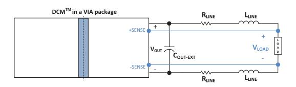
• Module performance is guaranteed for  $\Delta V_{OUT\_TO\_LOAD}$  within rated limits specified below. For  $\Delta V_{OUT\_TO\_LOAD}$  higher than the specified limits, regulation accuracy is not guaranteed. Also, high  $\Delta V_{OUT\_TO\_LOAD}$  might trigger OVP (for above nominal trim conditions), and might cause load voltage runaway (which might trigger UVP).
