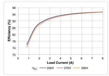
**Figure 5** — Efficiency at  $T_{CASE} = -55$ °C
