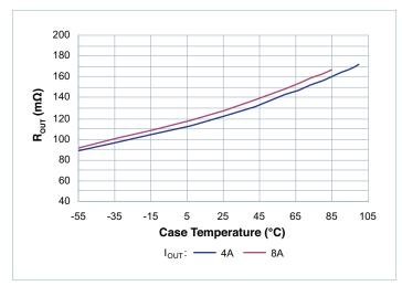
**Figure 13** — R<sub>OUT</sub> vs. temperature; nominal input
