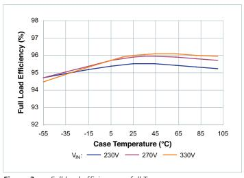
**Figure 3** — Full load efficiency vs. full  $T_{MAX}$  range
