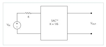
**Figure 21** — K = 1/6 Sine Amplitude Converter<sup>TM</sup> with series input resistor
