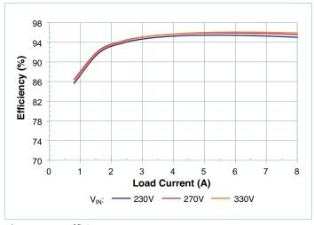
**Figure 9** — Efficiency at  $T_{CASE} = 85$ °C
