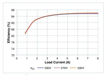
**Figure 7** — Efficiency at  $T_{CASE} = 25$ °C
