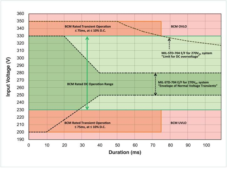
**Figure 19** — Envelope of normal voltage transient for 270V<sub>DC</sub> system.
