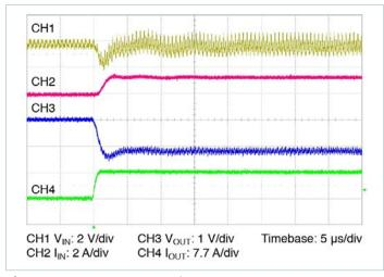
**Figure 17** — 0A - 8.00A transient response:  $C_{IN} = 100\mu\text{F}$ , no external  $C_{OUT}$
