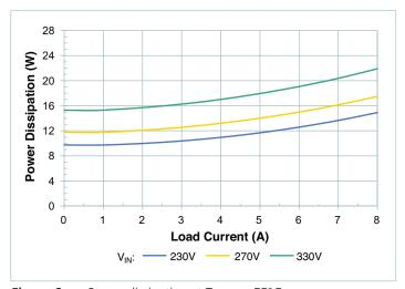
**Figure 6** — Power dissipation at T<sub>CASE</sub> = -55°C
