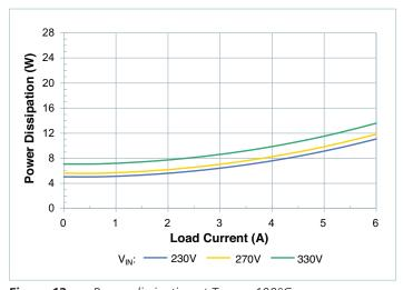
**Figure 12** — Power dissipation at  $T_{CASE} = 100$ °C
