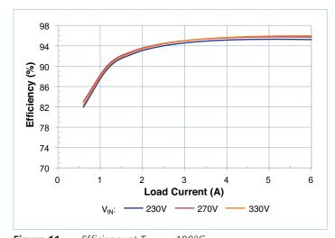
**Figure 11** — Efficiency at  $T_{CASE} = 100$ °C
