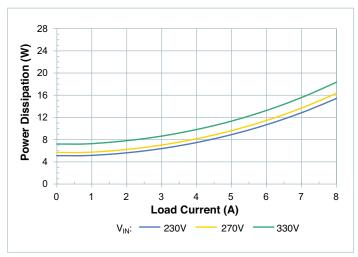
**Figure 10** — Power dissipation at  $T_{CASF} = 85$ °C
