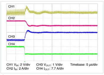
**Figure 18** — 8.00A - 0A transient response:  $C_{IN} = 100 \mu F$ , no external  $C_{OUT}$
