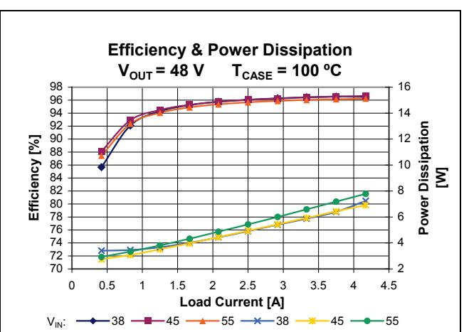
**Figure 10** – Total efficiency and power dissipation vs.  $V_{IN}$  and  $I_{OUT}$ ,  $V_{OUT} = 48\text{ V}$ ,  $T_{CASE} = 100\text{ }^{\circ}\text{C}$
