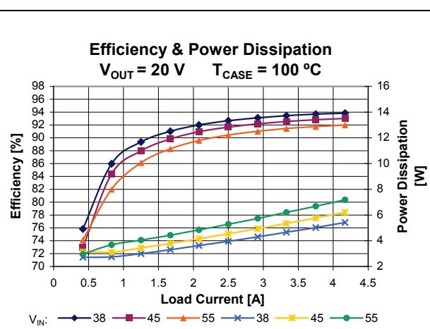
**Figure 9** – Total efficiency and power dissipation vs.  $V_{IN}$  and  $I_{OUT}$ ,  $V_{OUT} = 20\text{ V}$ ,  $T_{CASE} = 100\text{ }^{\circ}\text{C}$
