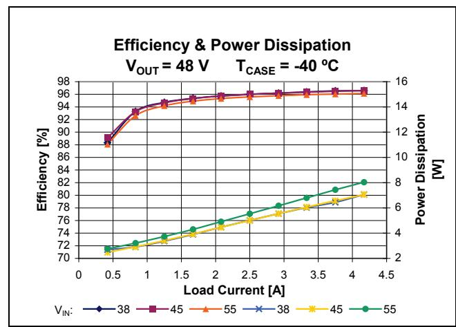
**Figure 4** – Total efficiency and power dissipation vs.  $V_{IN}$  and  $I_{OUT}$ ,  $V_{OUT} = 48 V$ ,  $T_{CASE} = -40^\circ C$
