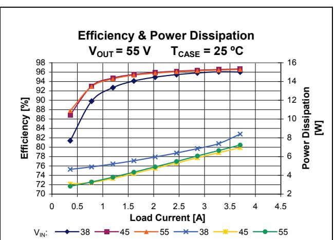
**Figure 8** – Total efficiency and power dissipation vs.  $V_{IN}$  and  $I_{OUT}$ ,  $V_{OUT} = 55\text{ V}$ ,  $T_{CASE} = 25\text{ }^{\circ}\text{C}$
