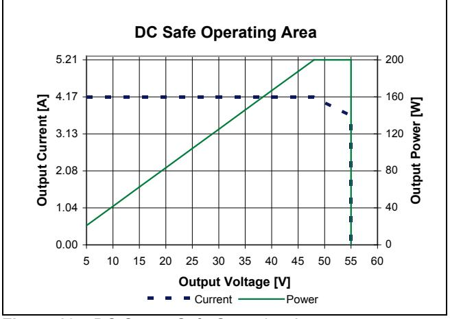
**Figure 16** – DC Output Safe Operating Area
