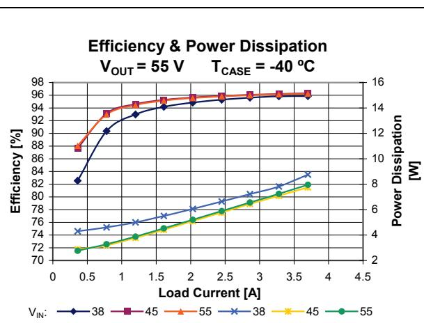
**Figure 5** – Total efficiency and power dissipation vs.  $V_{IN}$  and  $I_{OUT}$ ,  $V_{OUT} = 55\text{ V}$ ,  $T_{CASE} = -40\text{ }^{\circ}\text{C}$
