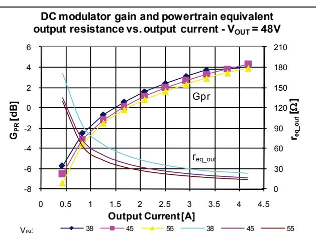
**Figure 19** – Powertrain characteristics vs.  $I_{OUT}$ ; Resistive load,  $V_{OUT} = 48$  V, various  $V_{IN}$
