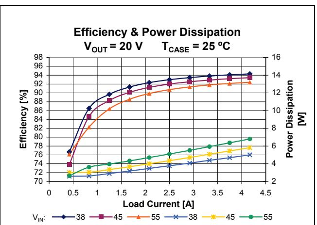
**Figure 6** – Total efficiency and power dissipation vs.  $V_{IN}$  and  $I_{OUT}$ ,  $V_{OUT} = 20\text{ V}$ ,  $T_{CASE} = 25\text{ }^{\circ}\text{C}$
