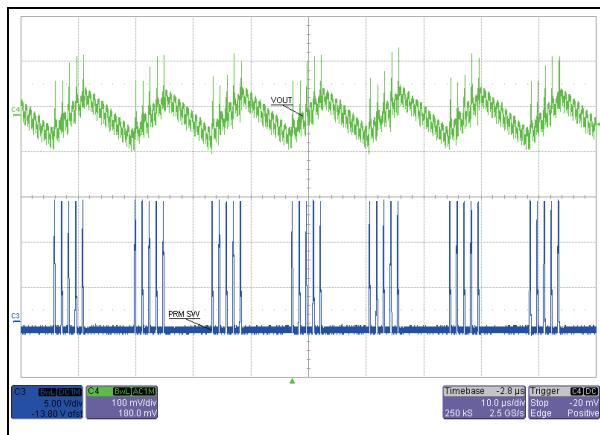
Figure 29 – light load burst mode of operation
