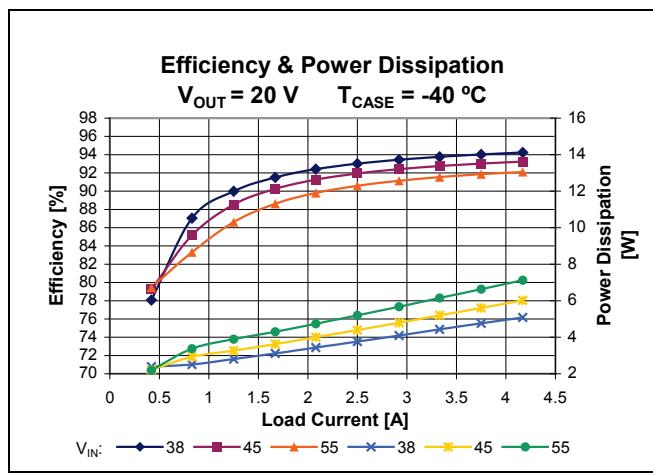
**Figure 3** – Total efficiency and power dissipation vs.  $V_{IN}$  and  $I_{OUT}$ ,  $V_{OUT} = 20 V$ ,  $T_{CASE} = -40^\circ C$
