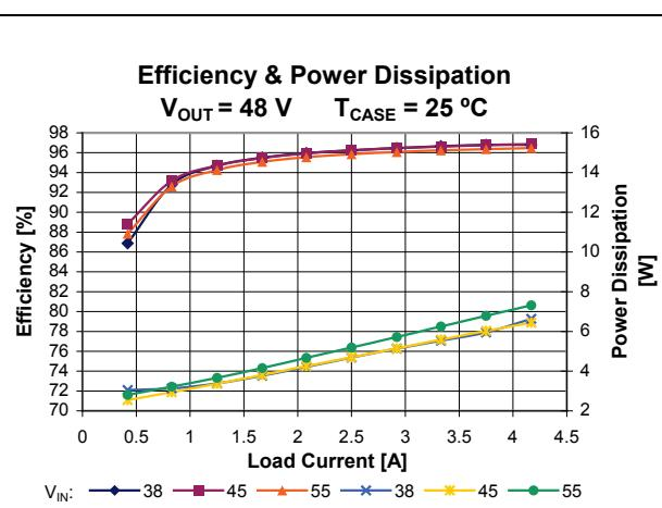
**Figure 7** – Total efficiency and power dissipation vs.  $V_{IN}$  and  $I_{OUT}$ ,  $V_{OUT} = 48\text{ V}$ ,  $T_{CASE} = 25\text{ }^{\circ}\text{C}$
