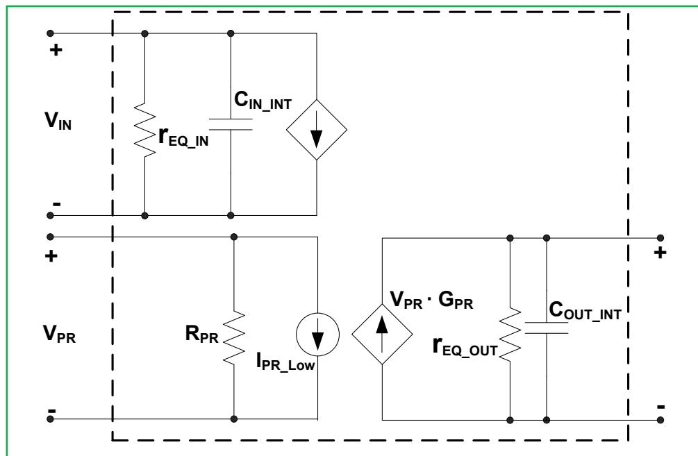
Figure 25 – PRM48BH480T200A00 AC small signal model
