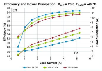
Figure 4 — Total efficiency and power dissipation vs.  $V_{IN}$  and  $I_{OUT}$  $V_{OUT} = 20.0 V$ ,  $T_{CASE} = -40^{\circ}C$
