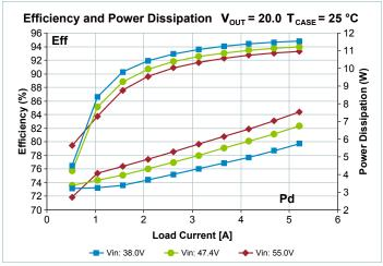
Figure 5 — Total efficiency and power dissipation vs.  $V_{IN}$  and  $I_{OUT}$  $V_{OUT} = 20.0 V$ ,  $T_{CASE} = 25^{\circ}C$
