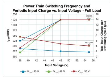
**Figure 14** — Typical Power Train Switching Frequency and Periodic Input Charge vs. V<sub>IN</sub>, V<sub>OUT</sub>; I<sub>OUT</sub> = 5.21 A
