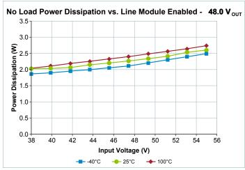
*Figure 2* — No Load Power Dissipation vs. V<sub>IN</sub>, module enabled
