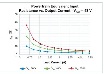
Figure 22 — Magnitude of powertrain dynamic input impedance vs.  $I_{OUT_{i}}$  $V_{INi}$ ,  $V_{OUT}$  = 48.0 V
