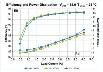
Figure 11 — Total efficiency and power dissipation vs.  $V_{IN}$  and  $I_{OUT}$  $V_{OUT} = 55.0 V$ ,  $T_{CASE} = 25^{\circ}C$
