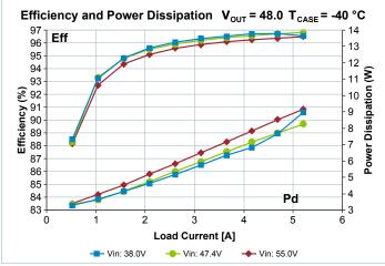
Figure 7 — Total efficiency and power dissipation vs.  $V_{IN}$  and  $I_{OUT}$  $V_{OUT} = 48.0 V$ ,  $T_{CASE} = -40^{\circ}C$
