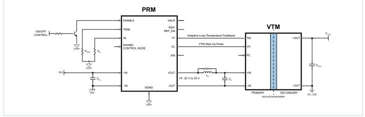
Figure 28 — PRM-VTM Adaptive Loop Example
