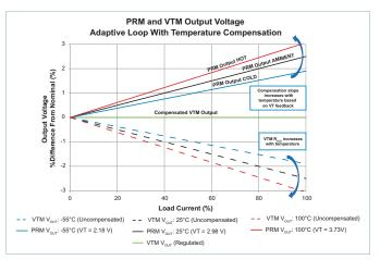
Figure 31 — Adaptive Loop Temperature Compensation Illustration
