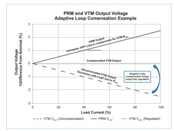
Figure 27 — Adaptive Loop Compensation Illustration
