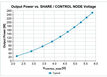
Figure 16 — Output Power vs. SHARE / CONTROL NODE Voltage;  $V_{IN} = 48.0 V$ ,  $V_{OUT} = 48.0 V$ ,  $T_{CASE} = 25^{\circ}C$
