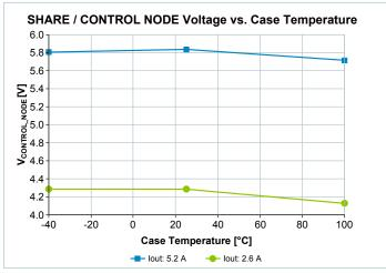
Figure 17 — Typical SHARE / CONTROL NODE Voltage vs.  $T_{CASE}$  and  $I_{OUT}$ ;  $V_{IN} = 48.0 V$ ,  $V_{OUT} = 48.0 V$
