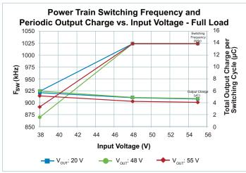
Figure 15 — Typical Power Train Switching Frequency and Periodic Output Charge vs.  $V_{IN_{*}}$   $V_{OUT}$ :  $I_{OUT} = 5.21$  A
