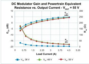
Figure 20 — Powertrain Characteristics vs.  $I_{OUT}$  V<sub>IN</sub> Resistive Load,  $V_{OUT} = 55.0 V$
