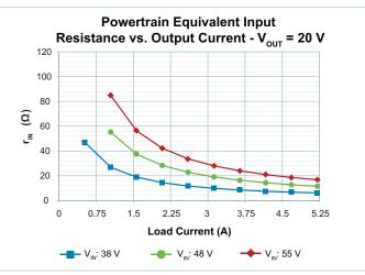
Figure 21 — Magnitude of powertrain dynamic input impedance vs.  $I_{OUT_i}$  $V_{INi}$   $V_{OUT} = 20.0$  V
