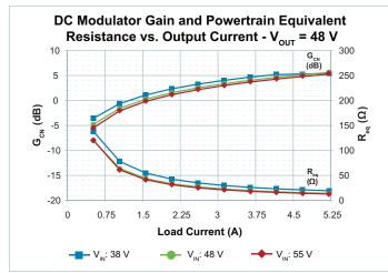
Figure 19 — Powertrain Characteristics vs. I<sub>OUT</sub>, V<sub>IN</sub> Resistive Load, V<sub>OUT</sub> = 48.0 V
