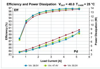
**Figure 8** — Total efficiency and power dissipation vs.  $V_{IN}$  and  $I_{OUT}$  $V_{OUT} = 48.0 V$ ,  $T_{CASE} = 25^{\circ}C$
