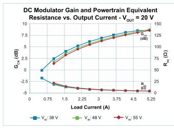
Figure 18 — Powertrain Characteristics vs.  $I_{OUT}$ ,  $V_{IN}$ Resistive Load,  $V_{OUT} = 20.0 V$
