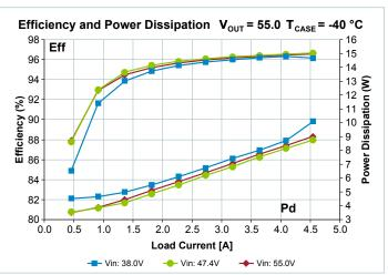
Figure 10 — Total efficiency and power dissipation vs.  $V_{IN}$  and  $I_{OUT}$  $V_{OUT} = 55.0 V$ ,  $T_{CASE} = -40^{\circ}C$
