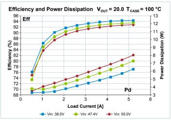
Figure 6 — Total efficiency and power dissipation vs.  $V_{IN}$  and  $I_{OUT}$  $V_{OUT} = 20.0 V$ ,  $T_{CASE} = 100^{\circ}C$
