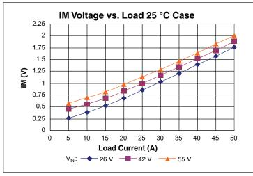
Figure 9 — IM voltage vs. load
