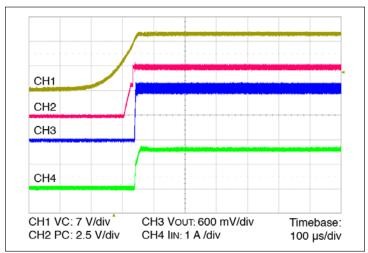
**Figure 14** — Start up from application of VC;  $V_{IN}$  pre-applied  $C_{OUT} = 0 \ \mu F$
