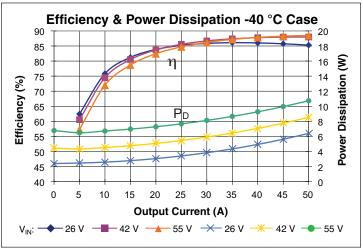
Figure 3 — Efficiency and power dissipation at -40°C
