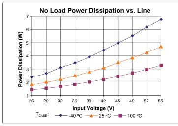
**Figure 1** — No load power dissipation vs.  $V_{IN}$
