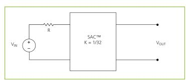
**Figure 18** — K = 1/32 Sine Amplitude Converter™ with series input resistor
