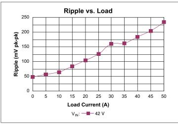
**Figure 7** — V<sub>RIPPLE</sub> vs. I<sub>OUT</sub>; No external C<sub>OUT</sub>. Board mounted module, scope setting: 20 MHz analog BW
