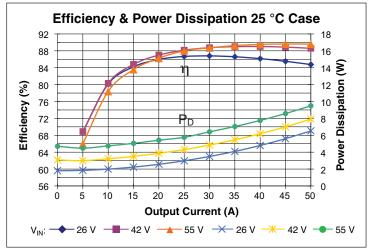
**Figure 4** — Efficiency and power dissipation at 25°C
