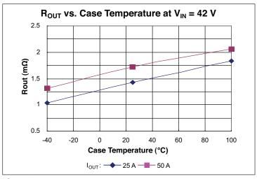
**Figure 6** — R<sub>OUT</sub> vs. temperature
