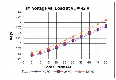
Figure 8 — IM voltage vs. load
