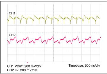
**Figure 12** — Full load ripple, 100  $\mu$ F C<sub>IN</sub>: No external C<sub>OUT.</sub> Board mounted module, scope setting : 20 MHz analog BW
