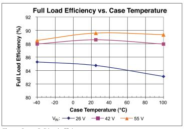
Figure 2 — Full load efficiency vs. temperature
