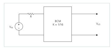
**Figure 20** — K = 1/16 BCM with series HI-side resistor
