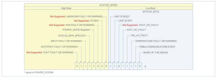
All fault or warning flags, if set, will remain asserted until cleared by the host or once the BCM and VDDB power is removed. This includes undervoltage fault, overvoltage fault, overvoltage warning, overcurrent warning, overtemperature fault, overtemperature warning, undertemperature fault, reverse operation, communication faults and analog controller shut-down fault.
