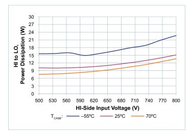
**Figure 4** — No-load power dissipation vs.  $V_{HI\_DC}$
