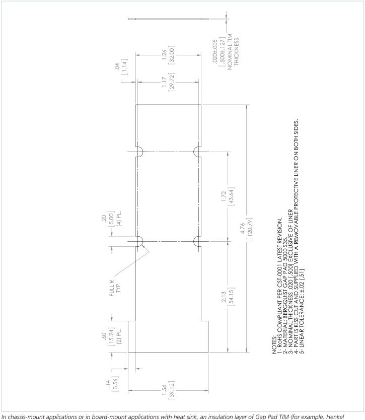
In chassis-mount applications or in board-mount applications with heat sink, an insulation layer of Gap Pad TIM (for example, Henkel Bergquist Gap Pad 5000S35 thickness 20 thousands, or similar) is necessary to meet the creepage requirements from the high-voltage terminals to the case. Vicor part number 45766 is the TIM Pad recommended for use with Vicor UHV BCM4414 VIA.
