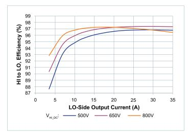
**Figure 6** — Efficiency at  $T_{CASE} = -55$ °C
