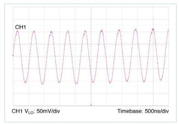
**Figure 14** — Full-load LO-side voltage ripple, no external C<sub>HI\_IN\_EXT</sub>; no external C<sub>LO\_OUT\_EXT</sub>. Board-mounted module, scope setting: 20MHz analog BW
