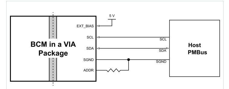
The controller of the BCM in a VIA package is referenced to the low-voltage-side signal ground (SGND).
