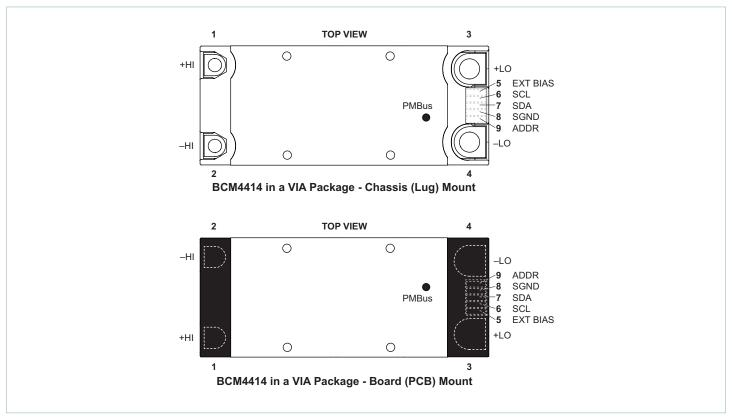
Note: The dot on the VIA housing indicates the location of the signal pin 9.
