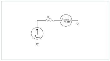
**Figure 23** — Single-sided cooling thermal model
