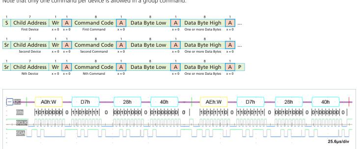
Figure 7 — DISABLE\_FAULT COMMAND (D7h)\_WRITE
