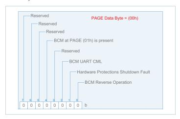
When the PAGE COMMAND (00h) data byte is equal to (00h), the BCM Reverse operation, Analog Controller Shut-Down Fault, and BCM UART CML bit will return the result of the active BCM. The BCM UART CML will also be asserted if the active BCM stops responding. The BCM must communicate at least once to the internal controller in order to trigger this FAULT. The BCM UART CML can be cleared using the PAGE (00h) CLEAR\_FAULTS (03h) Command.
