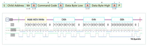
Figure 3 — TON\_DELAY COMMAND (D6h)\_WRITE WORD PROTOCOL
