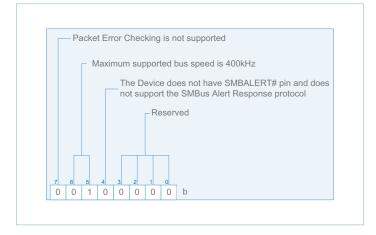
The BCM controller returns a default value of 20h. This value indicates that the PMBus® frequency supported is up to 400kHz and that both Packet Error Checking (PEC) and SMBALERT# are not supported.
