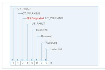
Unsupported bits are indicated above. A one indicates a fault.
