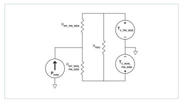
Figure 22 — Double-sided cooling thermal model
