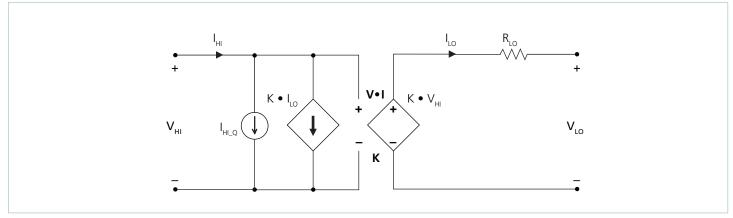
Figure 19 — BCM DC model (Forward Direction)
