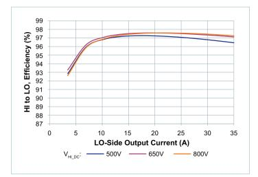
**Figure 10** — Efficiency at  $T_{CASE} = 70$ °C
