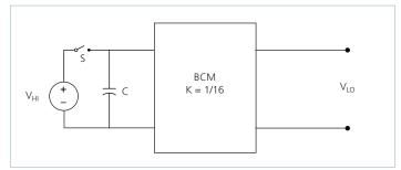
Figure 21 — BCM with HI-side capacitor
