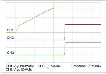
**Figure 17** — Start up from application of  $V_{HI\_DC}$  = 650V, 20%  $I_{LO\_DC}$  100%  $C_{LO\_OUT\_EXT}$
