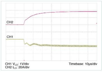
**Figure 15** — 0 – 35A transient response: no external  $C_{HI\_IN\_EXT}$  no external  $C_{LO\_OUT\_EXT}$
