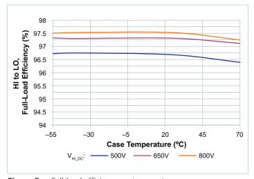
Figure 5 — Full-load efficiency vs. temperature
