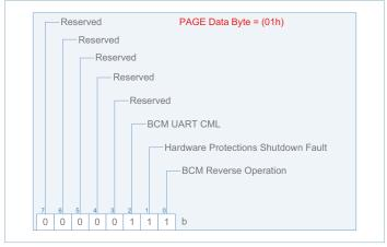
The reverse operation bit, if asserted, indicates that the BCM is processing current in reverse. Reverse current reported value is not supported.
