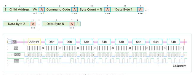
Figure 5 — SET\_ALL\_THRESHOLDS COMMAND (D5h)\_WRITE BLOCK PROTOCOL
