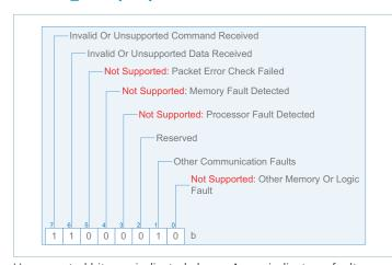
Unsupported bits are indicated above. A one indicates a fault. The STATUS\_CML data byte will be asserted when an unsupported PMBus® command or data or other communication fault occurs.
