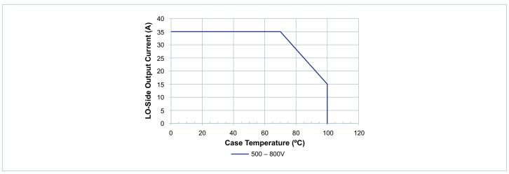
Figure 1 — Specified thermal operating area
