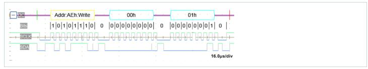
Figure 1 — PAGE COMMAND (00h), WRITE BYTE PROTOCOL
