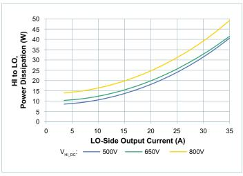
**Figure 11** — Power dissipation at  $T_{CASE} = 70^{\circ}C$
