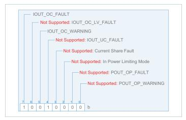
Unsupported bits are indicated above. A one indicates a fault.
