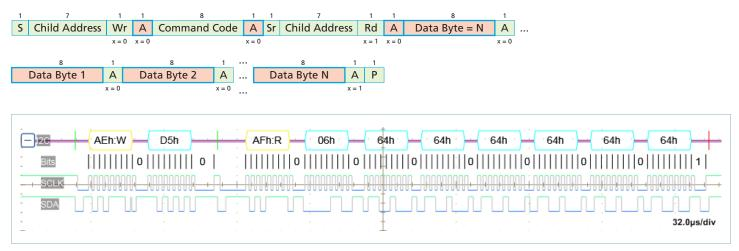
Figure 6 — SET\_ALL\_THRESHOLDS COMMAND (D5h)\_READ BLOCK PROTOCOL
