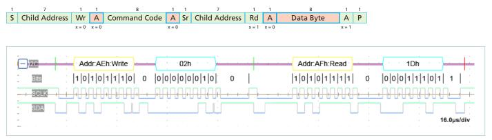
Figure 2 — ON\_OFF\_CONFIG COMMAND (02h), READ BYTE PROTOCOL
