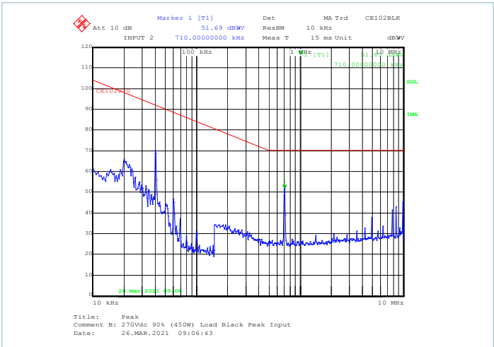
Figure 11 — Peak scan for the BLACK lead, 90% load
