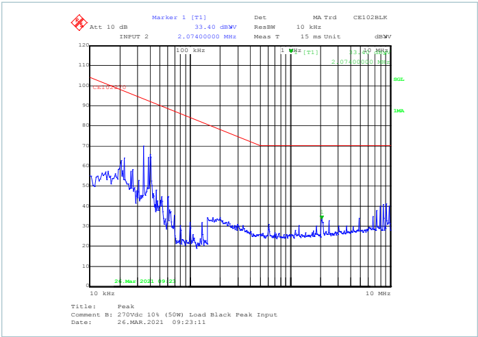
Figure 9 — Peak scan for the BLACK lead, 10% load
