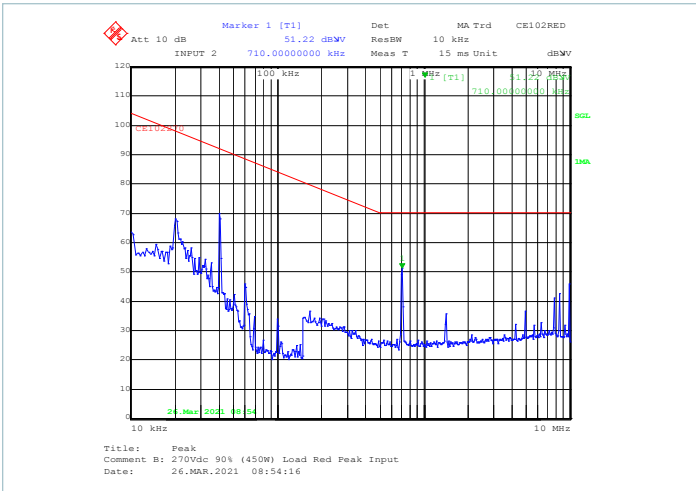
Figure 10 — Peak scan for the RED lead, 90% load
