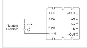
Figure 4 — LED on-state indicator
