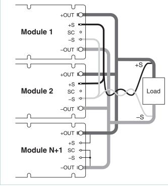
Figure 11 — N+1 module array output connections
