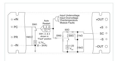
Figure 3 — PC/SC module alarm logic
