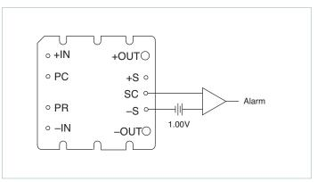
Figure 7 — Secondary-side on-state indicator
