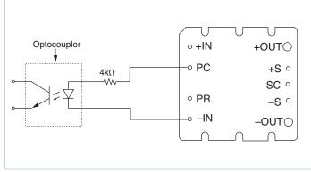
Figure 6 — Isolated on-state indicator
