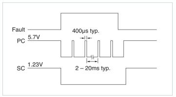
Figure 5 — PC/SC module alarm timing
