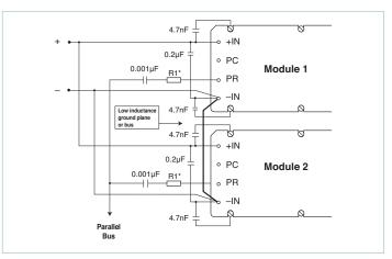
Figure 9 — AC-coupled single-wire interface \* See Maxi, Mini, Micro Design Guide
