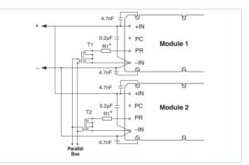
Figure 10 — Transformer-coupled interface
