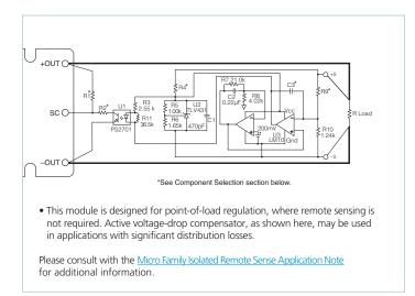
Figure 12 — Voltage-drop compensation
