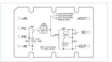
Figure 3 — PC/SC module alarm logic
