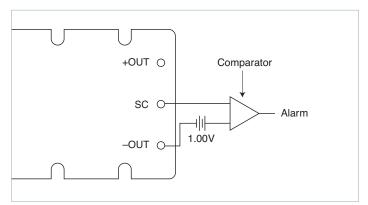
Figure 7 — Secondary-side on-state indicator
