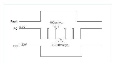
Figure 5 — PC/SC module alarm timing
