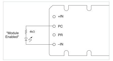
Figure 4 — LED on-state indicator
