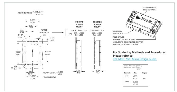
Figure 14 — PCB mounting specifications
