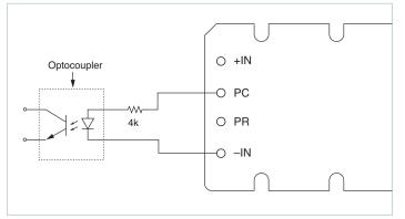
Figure 6 — Isolated on-state indicator
