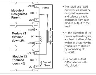
Figure 11 — N+1 module array output connections
