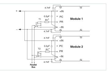
Figure 10 — Transformer-coupled interface
