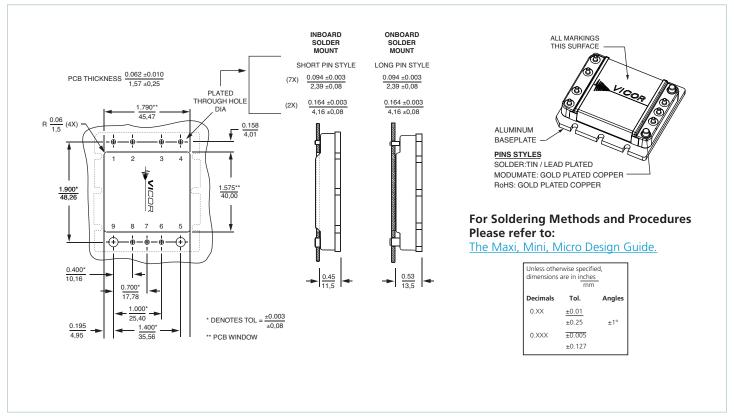
Figure 13 — PCB mounting specifications
