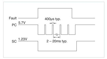
Figure 5 — PC/SC module alarm timing
