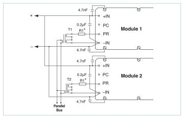
Figure 10 — Transformer-coupled interface
