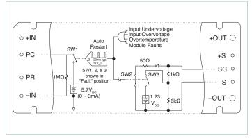
Figure 3 — PC/SC module alarm logic
