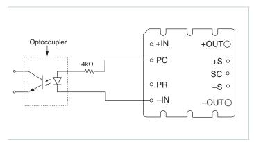
Figure 6 — Isolated on-state indicator
