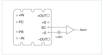
Figure 7 — Secondary-side on-state indicator
