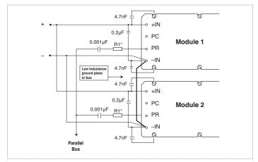
**Figure 9** — AC-coupled single-wire interface
