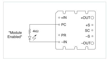
Figure 4 — LED on-state indicator
