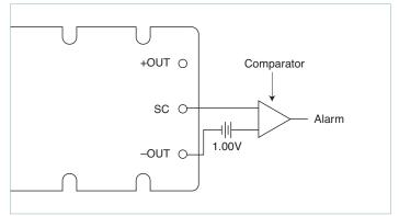
Figure 7 — Secondary side on-state indicator
