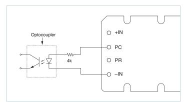
Figure 6 — Isolated on-state indicator
