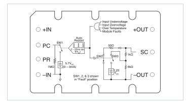
Figure 3 — PC/SC module alarm logic
