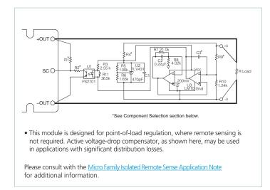
**Figure 12** — Voltage-drop compensation
