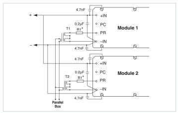
**Figure 10** — Transformer-coupled interface
