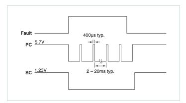
Figure 5 — PC/SC module alarm timing
