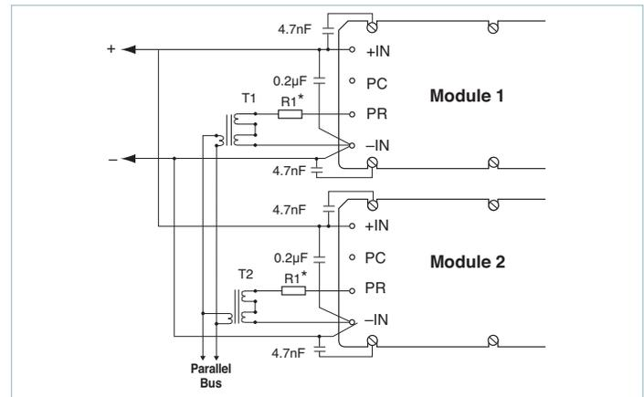
Figure 10 — Transformer-coupled interface
