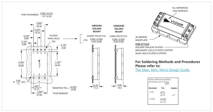
Figure 14 — PCB mounting specifications
