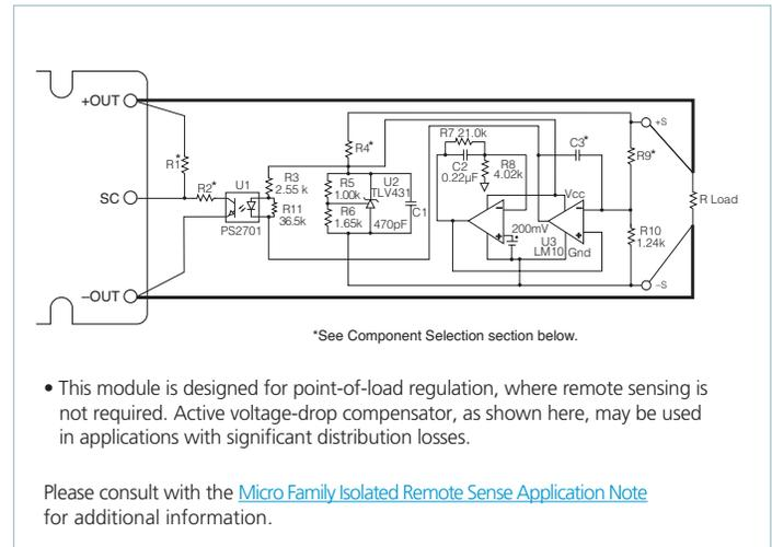
Figure 12 — Voltage-drop compensation
