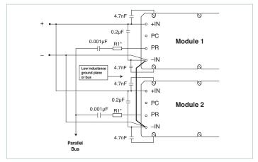
**Figure 9** — AC-coupled single-wire interface
