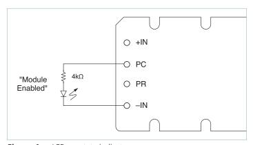
Figure 4 — LED on-state indicator
