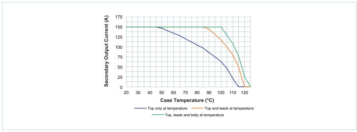
Figure 1 — Specified thermal operating area
