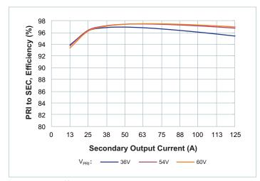
**Figure 10** — Efficiency at  $T_{CASE} = 80$ °C
