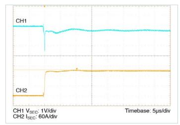
**Figure 15** — 0 – 150A transient response:  $C_{PRI\ IN\ EXT} = 2700\mu F$ , no external  $C_{SEC\ OUT\ EXT}$
