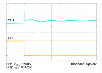
**Figure 16** — 150 – 0A transient response:  $C_{PRI\_IN\_EXT} = 2700\mu F$ , no external  $C_{SEC\_OUT\_EXT}$
