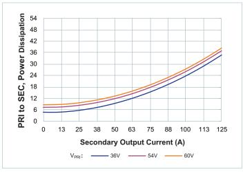
**Figure 11** — Power dissipation at  $T_{CASE} = 80$ °C
