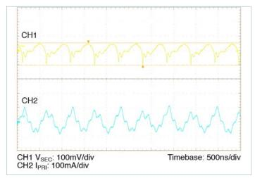
**Figure 14** — Full-load secondary voltage and primary current ripple, 2700μF C<sub>PRI\_IN\_EXT</sub>; no external C<sub>SEC\_OUT\_EXT</sub>. Board-mounted module, scope setting: 20MHz analog BW
