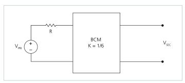
**Figure 20** — K = 1/6 BCM with series primary resistor
