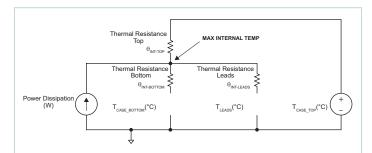
Figure 24 — Top case thermal model
