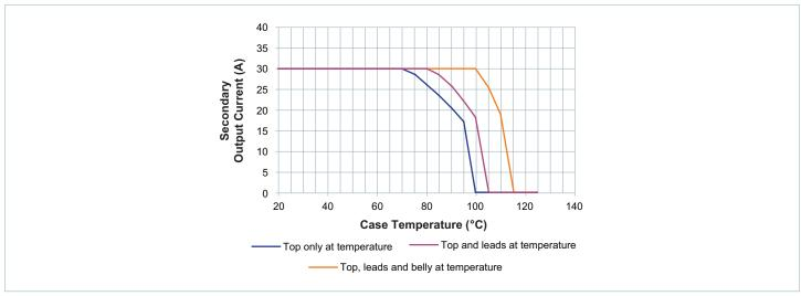
Figure 1 — Specified thermal operating area
