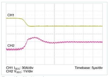
**Figure 16** — 30 – 0A transient response:  $C_{PRI\ IN\ EXT} = 10\mu F$ , no external  $C_{SEC\ OUT\ EXT}$
