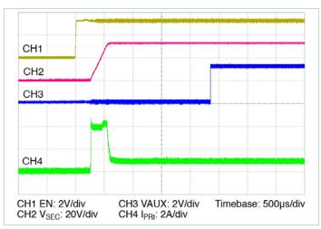
**Figure 18** — Start up from application of EN with pre-applied  $V_{PRI\_DC} = 270V$ ,  $20\% I_{SEC\_OUT\_DC}$ ,  $100\% C_{SEC\_OUT\_EXT}$
