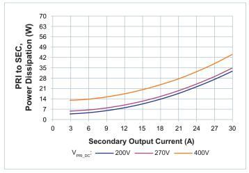
**Figure 11** — Power dissipation at  $T_{CASE} = 100$ °C
