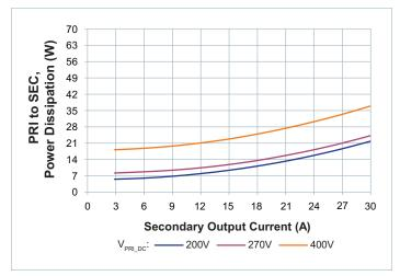
**Figure 7** — Power dissipation at  $T_{CASE} = -55$ °C
