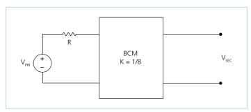
Figure 20 — K = 1/8 BCM with series primary resistor
