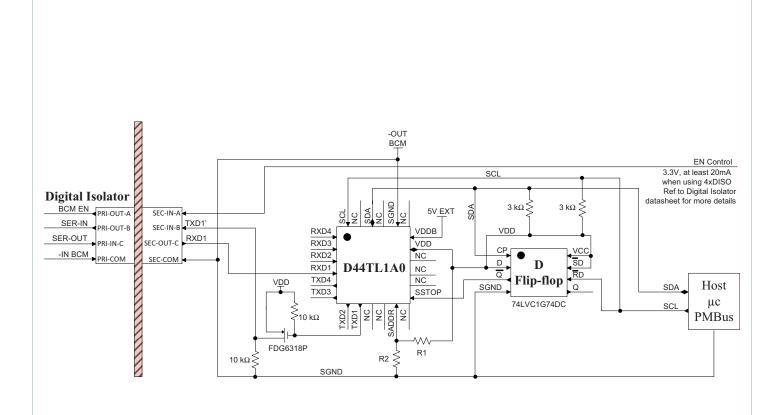
The PMBus communication enabled bus converter provides accurate telemetry monitoring and reporting, threshold and warning limits adjustment, in addition to corresponding status flags.
