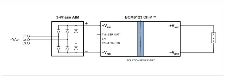
3-phase AC to point-of-load (3-phase AIM $^{TM}$  + BCM6123xD0G5030yzz)
