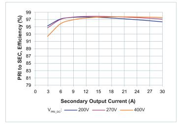
**Figure 8** — Efficiency at  $T_{CASE} = 25$ °C
