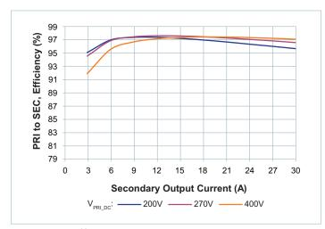
**Figure 10** — Efficiency at  $T_{CASE} = 100$ °C
