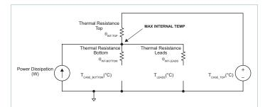
Figure 24 — Top case thermal model
