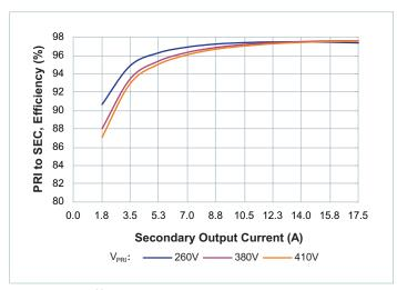
**Figure 6** — Efficiency at  $T_{CASE} = -40$ °C
