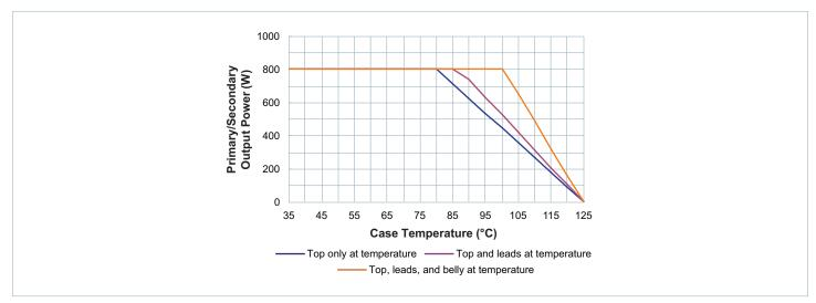
**Figure 1** — Specified thermal operating area
