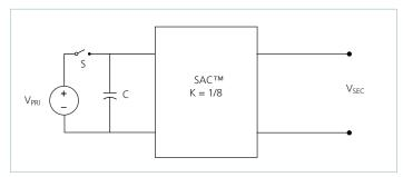
Figure 21 — Sine Amplitude Converter with primary capacitor
