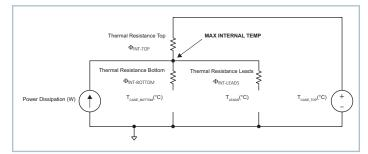
Figure 24 — Top case thermal model
