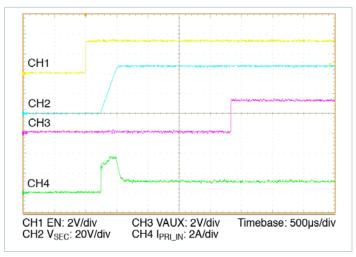
**Figure 18** — Start up from application of EN with pre-applied  $V_{PRI_DC} = 380V, 50\% I_{SEC_DC}, 100\% C_{SEC_OUT_EXT}$
