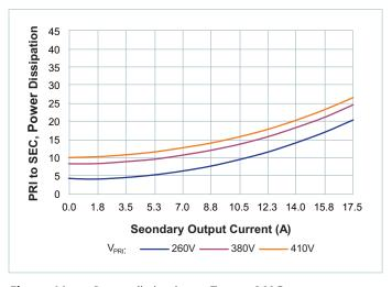
**Figure 11** — Power dissipation at  $T_{CASE} = 90^{\circ}C$
