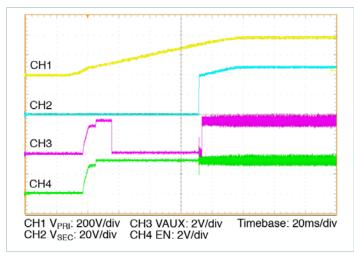
Figure 17 — Start up from application of  $V_{PRI\_DC}$  = 380V, 50%  $I_{SEC\_DC}$ , 100%  $C_{SEC\_OUT\_EXT}$
