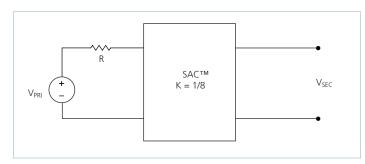
**Figure 20** — K = 1/8 Sine Amplitude Converter with series primary resistor
