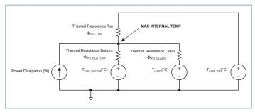
Figure 22 — Top case, Bottom case and leads thermal model
