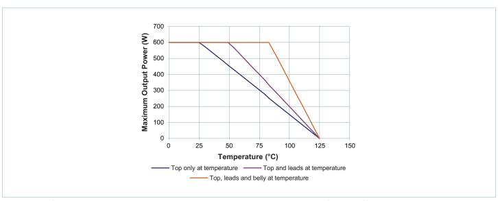
Thermal specified operating area: max output power vs. case temp, single unit at minimum full-load efficiency
