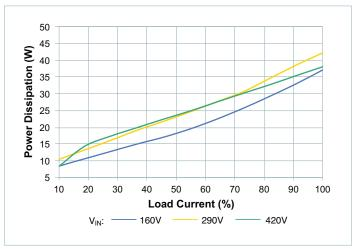
**Figure 14** — Power dissipation vs.  $V_{IN}$  to  $I_{OUT}$ ,  $T_{CASE} = 90$ °C
