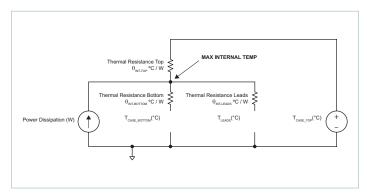
Figure 24 — One-side cooling thermal model
