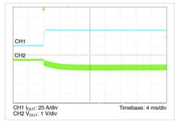
**Figure 16** — 10 – 100% load transient response,  $V_{IN}$  = 290V, nominal trim,  $C_{OUT\ EXT}$  = 1000 $\mu F$
