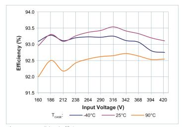
**Figure 7** — Full-load efficiency vs.  $V_{IN}$ ,  $V_{OUT} = 11.5V$
