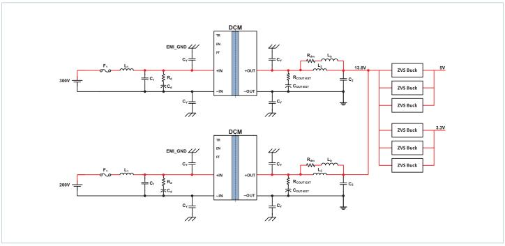
Typical application 2: DCM4623xC8G16F0yzz + ZVS Buck point-of-load
