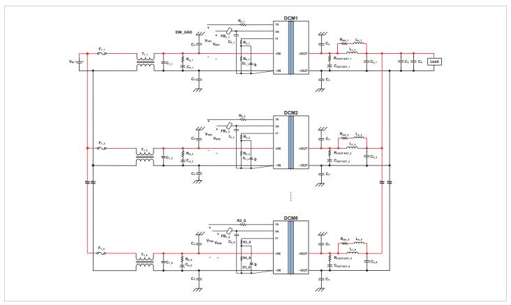
**Figure 26** — DCM paralleling configuration circuit 2
