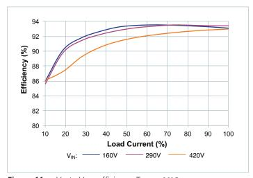
**Figure 11** —  $V_{IN}$  to  $V_{OUT}$  efficiency,  $T_{CASE} = 90^{\circ}$ C
