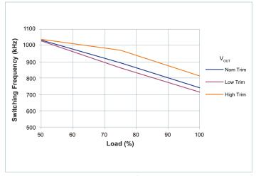
**Figure 20** — Powertrain switching frequency vs. load, at nominal  $V_{IN}$
