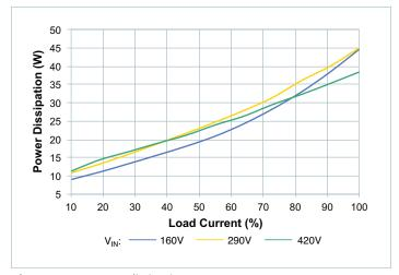
**Figure 15** — Power dissipation vs.  $V_{IN}$  to  $I_{OUT}$ ,  $T_{CASE} = 25$ °C
