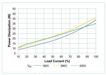
**Figure 13** — Power dissipation vs.  $V_{IN}$  to  $I_{OUT}$ ,  $T_{CASE} = -40$ °C
