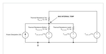
Figure 22 — Double-side cooling and leads thermal model
