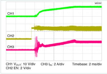
**Figure 6** — Initial start up from EN pin, with soft-start ramp.  $V_{IN} = 290V$ ,  $C_{OUT\ EXT} = 10000\mu\text{F}$ ,  $R_{LOAD} = 0.317\Omega$
