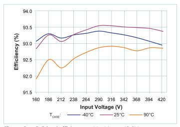
**Figure 8** — Full-load efficiency vs.  $V_{IN}$ ,  $V_{OUT} = 13.8V$
