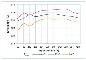
**Figure 9** — Full-load efficiency vs.  $V_{IN}$ ,  $V_{OUT} = 15.5V$
