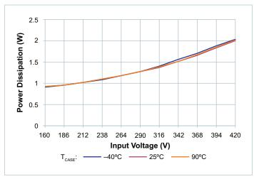
**Figure 2** — Disabled power consumption vs.  $V_{IN}$
