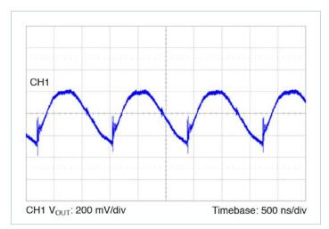
**Figure 21** — Typical output voltage ripple,  $V_{IN}$  = 290V,  $V_{OUT}$  = 13.8V,  $C_{OUT\_EXT}$  = 1000 $\mu$ F,  $R_{LOAD}$  = 0.317 $\Omega$
