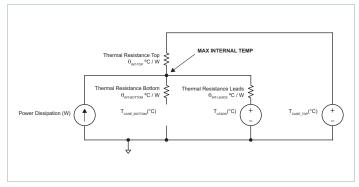
Figure 23 — One-side cooling and leads thermal model
