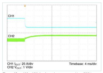
**Figure 19** — 100 – 10% load transient response,  $V_{IN}$  = 290V, nominal trim,  $C_{OUT\_EXT}$  = 1000 $\mu$ F
