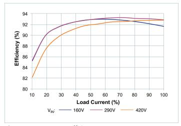
**Figure 12** —  $V_{IN}$  to  $V_{OUT}$  efficiency,  $T_{CASE} = 25^{\circ}C$
