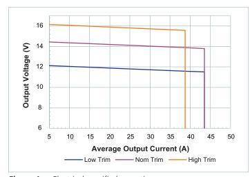
Figure 1 — Electrical specified operating area
