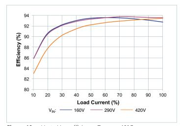
**Figure 10** —  $V_{IN}$  to  $V_{OUT}$  efficiency,  $T_{CASE} = -40$ °C
