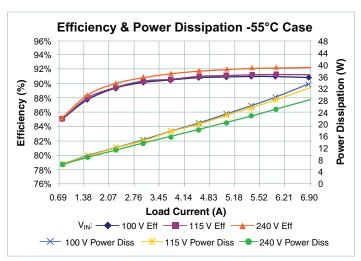
**Figure 19** —  $V_{IN}$  to  $V_{OUT}$  efficiency and power dissipation vs.  $V_{IN}$  and  $I_{OUT}$ ,  $T_{CASE} = -55^{\circ}\text{C}$
