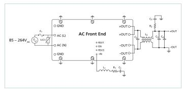
Figure 25 — Typical application for EN55022 Class B EMI
