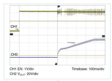
**Figure 9** — Typical start-up waveform, EN pin release,  $V_{IN}$  = 230V,  $R_{LOAD}$  = 7.1 $\Omega$ ,  $C_{OUT}$  = 6,800 $\mu$ F
