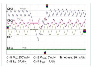
**Figure 11** — Line drop out, 50Hz, 90° phase,  $V_{IN}$  = 230V,  $P_{LOAD}$  = 330W,  $C_{OUT}$  = 6,800 $\mu$ F
