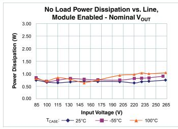
**Figure 3** — Typical no-load power dissipation vs.  $V_{IN}$ , module enabled
