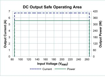
Figure 1 — DC output safe opearating area
