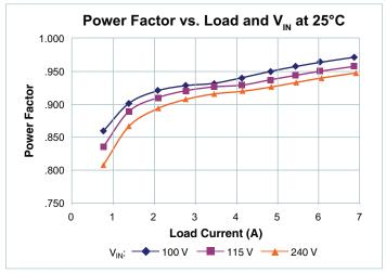
**Figure 18** — Typical power factor vs.  $V_{IN}$  and  $I_{OUT}$
