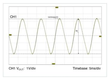
**Figure 6** — Typical line frequency output voltage ripple waveform,  $T_{CASE} = 30$  °C,  $V_{IN} = 230V$ ,  $I_{OUT} = 6.9$ A,  $C_{OUT} = 6,800\mu$ F. Measured at C3, Figure 25
