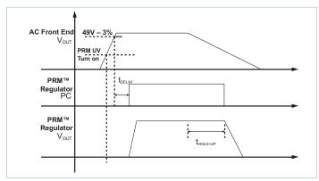
Figure 27 — PRM enable hold-off waveforms
