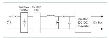
Figure 24 — Traditional PFC AC-to-DC supply
