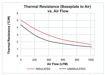
**Figure 22** — Baseplate-to-air thermal resistance; Insulated: minimal thermal dissipation through pins to PCB;
