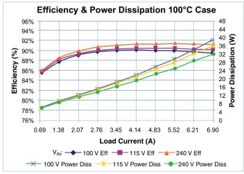
**Figure 21** —  $V_{IN}$  to  $V_{OUT}$  efficiency and power dissipation vs.  $V_{IN}$  and  $I_{OUT}$ .  $T_{CASE} = 100$ °C
