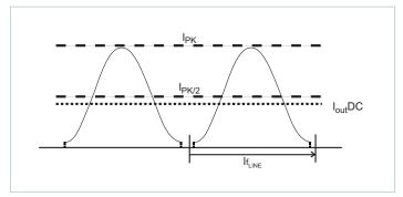
Figure 26 — Output current waveform
