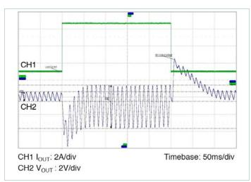
**Figure 7** — Typical output voltage transient response,  $T_{CASE} = 30^{\circ}\text{C}$ ,  $V_{IN} = 230V$ ,  $I_{OUT} = 6.9A$ ,  $C_{OUT} = 6,800\mu\text{F}$
