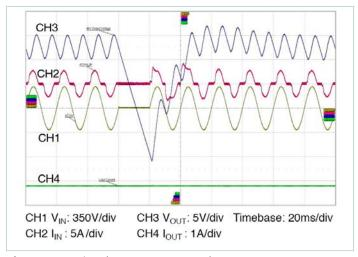
Figure 10 — Line drop out, 50Hz, 0° phase,  $P_{LOAD} = 330W$ ,  $C_{OUT} = 6,800\mu F$
