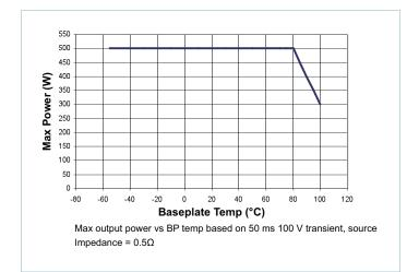
Figure 5 — Temperature de-rating
