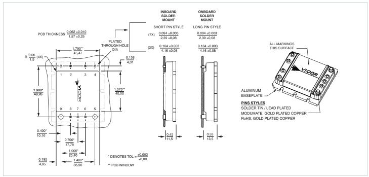
Figure 9 — PCB mounting specifications
