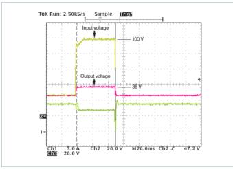
Figure 1 — Transient immunity: M-FIAM9 output response to an input transient
