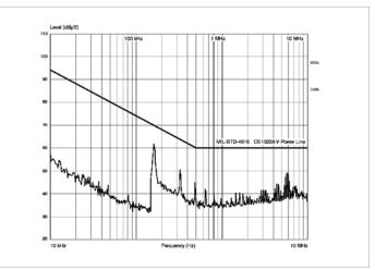
Figure 2 — Conducted noise: M-FIAM9 and model V28A12M200B DC-DC converter operating at 28V<sub>DC</sub>, 200W
