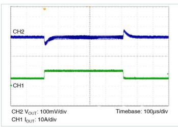
Figure 4 — Transient response: 7.5 – 15A, at 5A/µs
