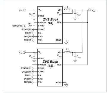
*Figure 16* — *PI34xx-00 parallel operation*
