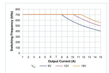
Figure 3 — Switching frequency vs. load current
