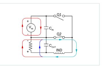
Figure 22 — Current flow: Q2 closed
