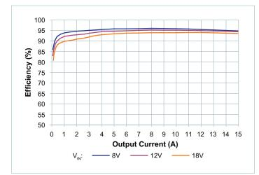
Figure 1 — Efficiency at 25°C
