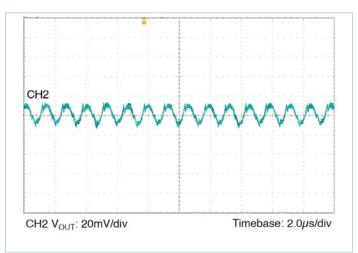
Figure 12 — Output ripple  $12V_{IN}$  5.0 $V_{OUT}$  at 7.0A;  $C_{OUT} = 8 \times 47 \mu F$
