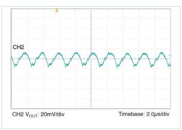
Figure 5 — Output ripple  $12V_{IN} 3.3V_{OUT}$  at 15A;  $C_{OUT} = 8 \times 100 \mu F$
