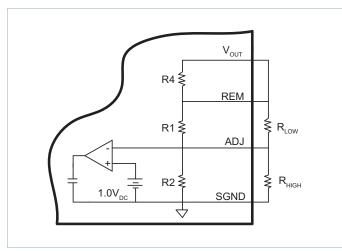
Figure 17 — Internal resistor divider network
