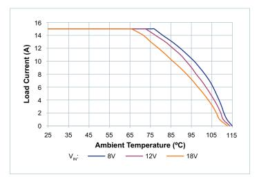
Figure 14 — PI3424 – load current vs. ambient temperature, OLFM
