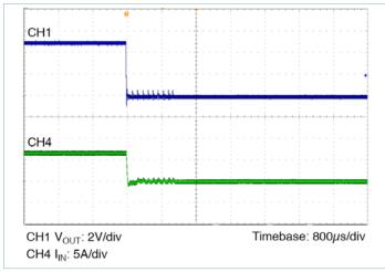
Figure 8 — Short circuit test
