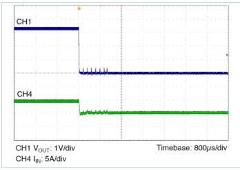
Figure 2 — Short circuit test
