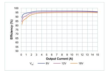
Figure 7 — Efficiency at 25°C
