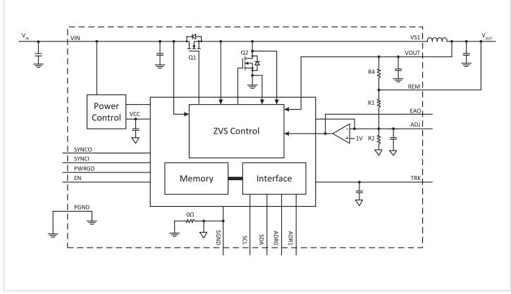
Simplified block diagram (I<sup>2</sup>C<sup>™</sup> pins SCL, SDA, ADR0, and ADR1 are for factory use only. Not for use in application.)
