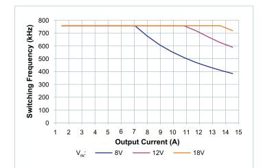
Figure 9 — Switching frequency vs. load current
