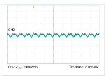
Figure 6 — Output ripple  $12V_{IN} 3.3V_{OUT}$  at 7.0A;  $C_{OUT} = 8 \times 100 \mu F$
