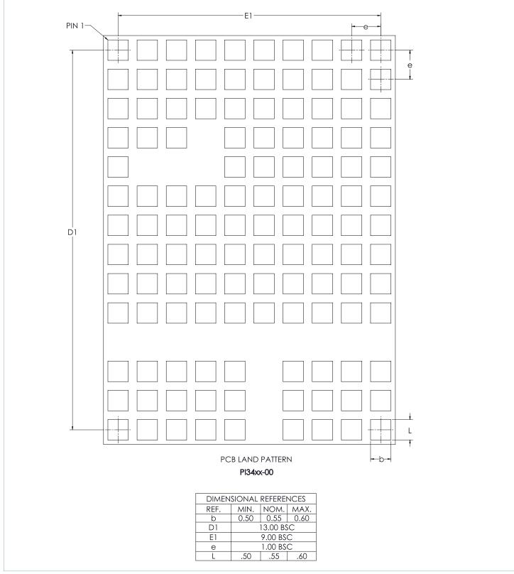
Recommended receiving footprint for PI34xx-00 10 x 14mm package. All pads should have a final copper size of 0.55 x 0.55mm, whether they are solder-mask defined or copper defined, on a 1 x 1mm grid. All stencil openings are 0.45mm when using either a 5 or 6mil stencil.
