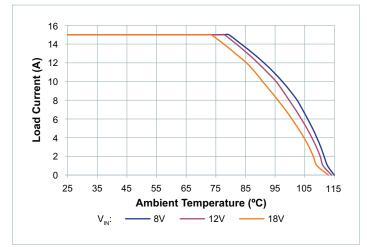
Figure 13 — PI3423 – load current vs. ambient temperature, OLFM
