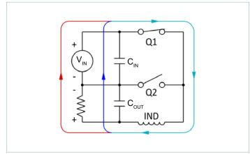
Figure 21 — Current flow: Q1 closed
