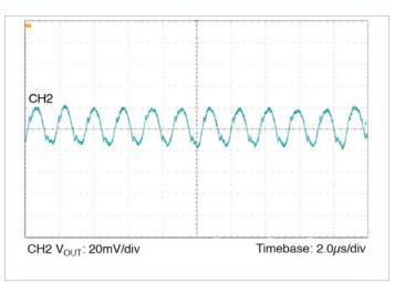
Figure 11 — Output ripple  $12V_{IN} 5.0V_{OUT}$  at 15A;  $C_{OUT} = 8 \times 47\mu F$
