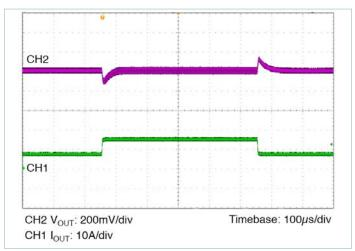
Figure 10 — Transient response: 7.5 – 15A, at 5A/µs
