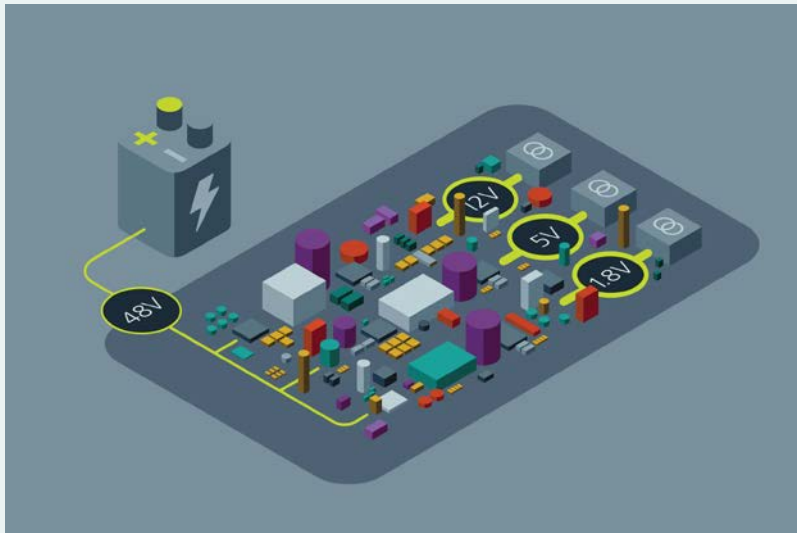
Figure 3: Discrete solutions have more components to manage which increases design complexity.
