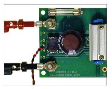
Figure 7: PR transformer and isolated PR bus
