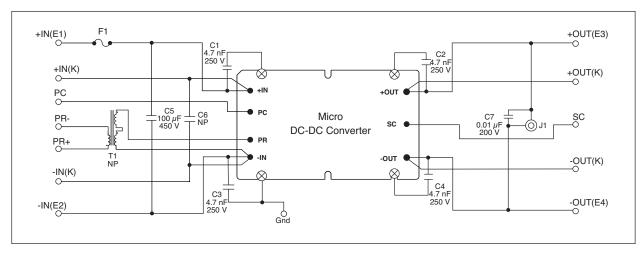
Figure 5: Micro DC-DC converter Evaluation Board schematic
