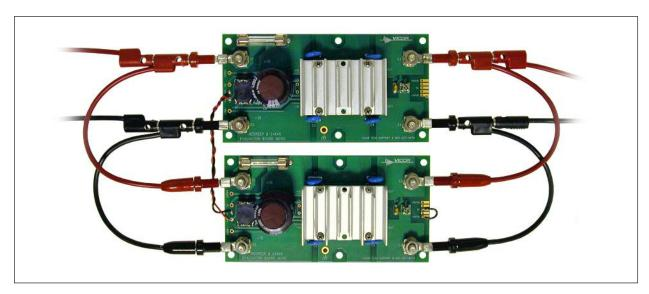
Figure 6: Paralleled Evaluation Board, wire gage is suitable for high input and output voltage converters
