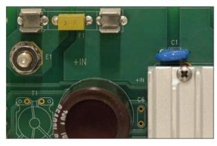
Figure 4: Fuse installation for PC-Tron
