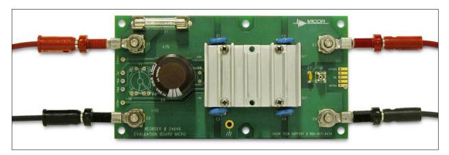
Figure 2: Basic Evaluation Board connections, high voltage input and output
