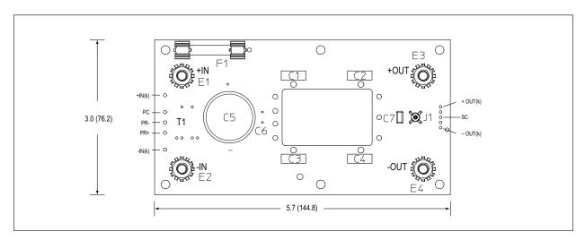
Figure 1: Micro Evaluation Board layout and dimensional drawing, component side.
