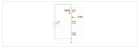
The charging current can be adjusted by changing R104 per the following equation.
