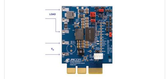
Install: JISP, JISN connecting RSENSE to IS+ and IS-, J200 connecting IMON to LGH, JTRK.
