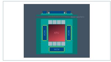
Figure 2 – Lateral power delivery has typical resistance of 70  $\mu\Omega$  and a PDN loss at 1,000A of 70W
