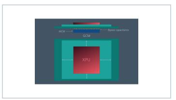
**Figure 3** – Vertical power delivery has typical resistance of 10  $\mu$ Ω and a PDN loss at 1,000A of 10W 70W
