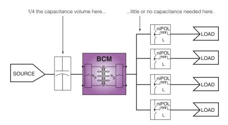
BCMs are also available with high voltage (352 V, 384 V) input capabilities for high density DC-DC conversion, typically following a PFC stage in offline AC-DC conversion down to 48 V or 12 V.
