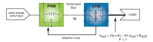
Under remote loop control, illustrated in Fig. 9, the voltage at the load is sensed and fed back to the PRM. This feedback protocol provides the most accurate load regulation - within +/- 0.2% - but may require isolation in the feedback path.
