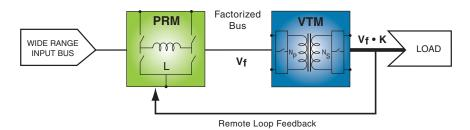
With the addition of a (PI1004) Picor point-of-load IC, remote loop control can incorporate a digital control option compatible with the latest processor VID specifications.
