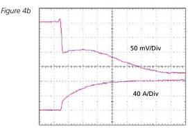
0-80 A Load step with 100  $\mu F$  output capacitance
