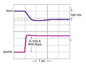
The VTM's high bandwidth obsoletes the need for massive point-of-load bypass capacitance. Even without any external output capacitors, the output of a VTM® exhibits a limited voltage perturbation in response to a sudden power surge. A minimal amount of external bypass capacitance, in the form of low ESR/ESL ceramic capacitors, suffices to eliminate any transient voltage overshoot.
