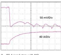
0 – 80 A Load step with NO output capacitance
