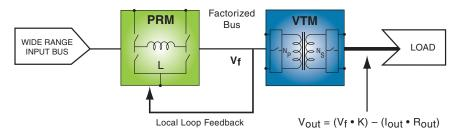
Under adaptive loop control, illustrated in Fig. 8, the VTM sends a signal back to the PRM to enable the PRM to adjust the Factorized Bus Voltage to compensate for the VTM output resistance. Adaptive loop control provides improved regulation over the simple local loop control – within +/- 1% – yet requires only a simple, non-isolated, feedback connection between the VTM and PRM.
